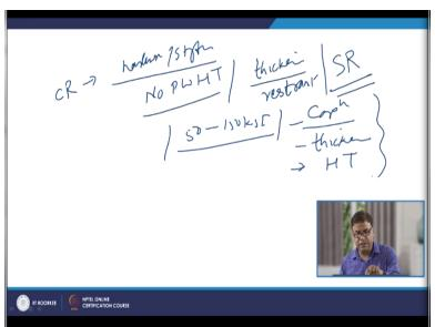
Generally the fusion welding of first the cooling rates which results in the reasonable good hardness and strength of the weldment. And that is why generally no post weld heat treatment after the welding is needed with these steels except when very thick sections are being welded. And the welding is being carried out under restrain conditions in those cases the stress reliving heat treatment is carried out.
