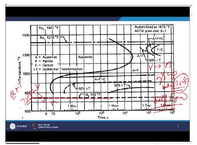
So, if we see there are 2 or 3 zones about which we can say like what happens to the steel when it is exposed constant temperature in range of 1100 degree Fahrenheit to 1300 degree Fahrenheit this is one zone. Then another zone is 950 to the 1100 Fahrenheit and what happens when steel is exposed at a temperature below 950 degree centigrade. So the responses of the Q and T steels when of the 517 or 514 type when it is given exposure at a constant temperature for longer time.
