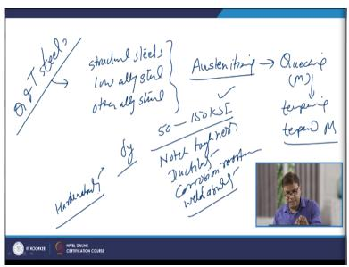
These are basically quenched and tempered steels, so these steels are basically how these are realized these can be the structural steels. These can be low alloy steels and these can be other alloy steel category. These steels are basically developed means Q and T steels can be of these categories which are developed following sequence of heat treatment involving austenitizing means we have to heat it, so that homogeneous austenite is formed followed by quenching.
