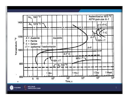
So, as per the micro constituents there will be different amount of the as per the composition and the kind of heat treatment which is being given. The steels may have the different micro constituents primarily these are design to have the bainite and martensite. But if the there are certain compositions where it can have the ferrite, bainite and the martensite. So, as per the kind of the heat treatment conditions and the tempering conditions which are being imposed.
