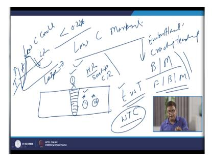
Most of these steels are actually designed to have the low carbon content which is less than 0.22%. So that whatever martensite is found that is of the low carbon martensite and it does not lead to the much of the embrittlement or increase in cracking tendency. So cracking tendency and the embrittlement tendency both are reduced because of the low carbon martensite formation.
