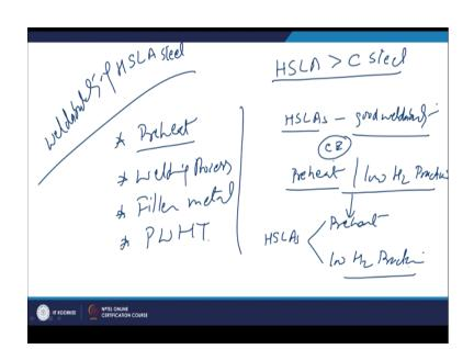
Now if you talk of the typical details related with the weldability of high strength low alloy steels then you need to talk about the 4 different aspects one is like the kind of preheat which is to be used during the welding of the HSLAs then what welding processes can use and what are the issues related with then what kind of the filler metal we can use and what other options available for welding the different category of the or different types of high strength low alloy steels.
