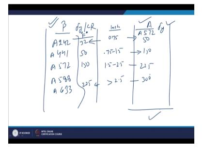
So the heat expansion during the heating and subsequent contraction can be more problematic with regard to the cracking tendency. So I have set there are 2 broad groups of the HSLAs the group B is primarily for the high yield strength as well as corrosion resistance and group A is mainly for high yield strength steels like when the plates of the different thicknesses are welded of say up to 0.75 inch.
