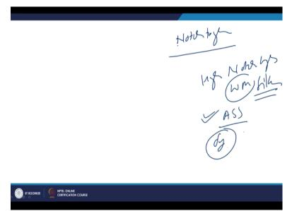
Then we may choose the high notch toughness weld metal fillers, the fillers which will provide the higher notch toughness, so like ASS can be used for welding of the HSLAs provided other strength requirements like yield strength requirements are satisfied because this will provide very good the resistance to the a notch toughness.
