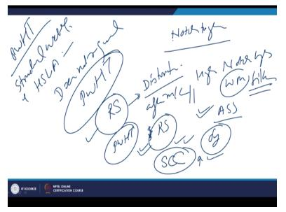
And normally in structural welding, so PWHT post weld heat treatment structural welding of HSLAs does not require PWHT post weld heat treatment is normally not required for most of the structural welding of the high strength low alloy steel weld joints. But we know that whenever the steels are welded these invariably developed the residual stresses. So presence of the residual stresses swill be increasing the tendency for distortion especially after machining.
