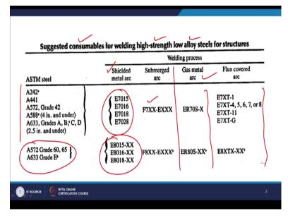
Now we will see there is a like the different fillers and the consumables which are used for welding of the high strength low alloy steels used for joining of the various structural components. So the different grades of the HSLAs when they are welded using the shielded metal arc welding, these are the set of the electrodes most of these are the low hydrogen electrodes of the 7000 series.
