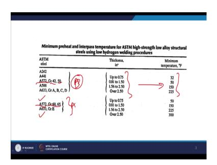
The structure is in general finder for the HSLAs as compared to that of the carbon steel and what this table shows that the kind of the minimum preheat which is to be used as I said this is a group A HSLAs for different thicknesses we need the different magnitude of the preheat ranging from 32 to 25 for sorry for group B steels and for group A steel we are like 572 and 633. The other different sub grades of because we have 572 here and 572 here as well.
