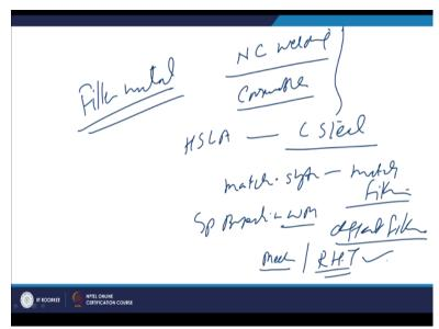
As far as the filler is concerned filler metal, some of the welding process of the non consumable welding processes and there are few consumable welding processes. So the line are the criteria for selection of the filler metal for HSLAs is similar to that of the carbon steels like for matching strength we choose the matching filler, but if we require some specific property in the weld metal then different filler is chosen.
