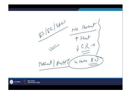
Now will see that since the electro slag and electro gas and SAW which is performed using very high heat input we do not require any preheat because these processes are of the so high heat input that cooling rate is no enough in order to facilitate the formation of the softer phases and sometimes even the phases are so soft and so course that they deteriorate the notch toughness and the mechanical properties of the metal.
