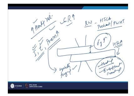
And after the heating the force is applied followed by the cooling at a very high rate. So the heating rate and the cooling rates both are high with when the resistance welding processes are used for welding of the HSLAs say resistance welding process like the spot welding or the same welding when it is used so in that case since these are of the high yield strength processes and the resistance for the flow of current is almost same as that of the carbon steels.
