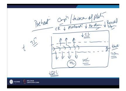
So whenever we use a preheat of course for the preheat will be the function of the composition and thickness of the plate of the section thickness which is to be welded, whenever we apply preheat it helps to reduce like these are the plates this is the weld centre line. So the preheating is to be done with minimum up to the distance means from the distance up to which preheating should be done will be equal to the thickness of the plate are 75 mm whichever is larger.
