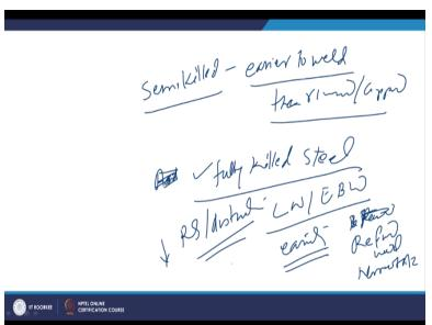
So as far as the semi killed steels are concern these are somewhat easier to weld by the laser and electron beam welding then the rimmed and capped steels. So for these advanced welding processes these advanced welding process like laser and radiation, laser and electron beam processes it will be better to use the fully killed steels. So when the fully killed steels are subjected to the laser welding or electron beam welding.
