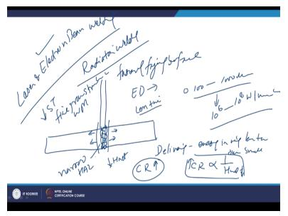
Apart from that if you get time then we will talk about the high strength a low alloy steels. So we know that the laser and electron beam, both these welding processes are known as the radiation welding process because the radiations in form of the laser and the electron beam are used for fusion of the faying surfaces of the metal to be joined and the energy density which is associated with these sources which have the capability to apply the energy over a very small area.
