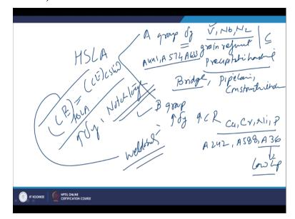
And this equation can be used to calculate the carbon equivalent for HSLAs high strength low alloy steels. Now there are all HSLAs are grouped in three 2 broad categories 1 is like high strength low alloy Steels that 2 broad groups is A group, group A is steels are primarily designed for high yield strength and this is realized with the addition of the vanadium, niobium and/or either singly or in combination or sometimes nitrogen is also added in very controlled way.
