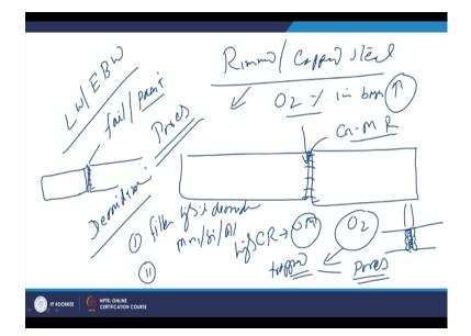
So as far as the laser welding or electron beam welding of the rimmed and capped steels are concerned which are not actually deoxidized for retaking care of the oxygen contents, so the oxygen percentage in the base metal is very high and because of this when the seats or the plates to be welded either of the low carbon, medium carbon, high carbon or mild steel. They will be leading to the removal of the oxygen very violent gas metal reactions will be taking place due to the release of oxygen.
