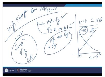
Now we talk about so this is where we complete about the weldability aspects of the carbon steels, now will take up the some introduction aspects of the high strength, low alloy steel. So this classification is primarily based on the, this classification of the steel is based on the mechanical properties where these are designed for high strength. So high strength, low alloy steels. These are design primarily for the high yield strength.
