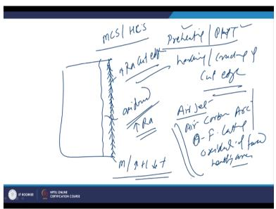
So as far as the mild steel and low carbon steel is concerned there is no hardenability issue and it can be cut easily soon, cutting is easy in case of the mild steel and the low carbon steels but if it is the medium carbon steel or high carbon steel then just like welding we need to take care of proper heating and the post heat treatment. So that unnecessary hardening and cracking of cut age can be reduced h.
