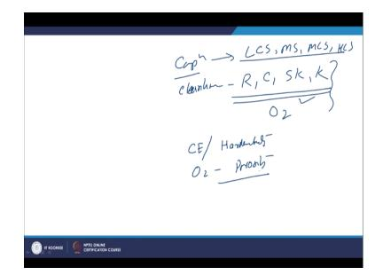
So this is the main aspect as far as the laser and electron beam welding is concerned, **so** but with the steels we have our in terms of the composition, in terms of the cleanliness like we may have the low carbon steel, mild steel, medium carbon steel, high carbon steel likewise rimmed steel, capped steel, semi killed steel or the killed steel. So different compositions, different purity level with regard to the oxygen as far as the cleanliness is concerned.
