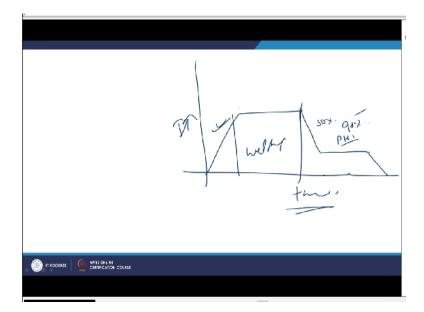
In more simplified form what we say that the current is increased then it is held. Then, so this is the welding time and then current is reduced then again the current is supplied. So, current is reduced then the current is maintained at a certain level. So, that post heat treatment can be performed and then it is again reduced. So, now this level of the current to be used may be 50%-90% of the welding current which is being used for the welding purpose.
