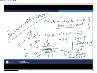
In case of the resistance welding processes, the most common welding process are like spot welding, seam welding, projection welding, and high frequency resistance and induction welding. Then we have this is called high frequency may be resistance welding and the flash welding which is mostly flash butt welding. So these are most common resistance welding processes and like the projection, seam.
