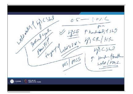
So, which are used now if we see the weldability of the high carbon steel. High carbon steel actually has the carbon content in the range of 0.5-1%. So, such a high level of the carbon content coupled with the manganese leads to the very high carbon equivalent. High carbon equivalent causes significant increase in the hardenability of the steel and the high cooling rate.
