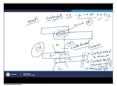
And therefore it becomes crucial that if the sheets which are being joined or having the medium or high hardenability then the cooling rate becomes crucial with regard to the austenite to martensitic transformation increase in hardness, increase in cracking tendency. So we need to be more careful with regard to the cooling rate being experienced by the weld nugget and heat affected zone during the spot welding of those steels having the some good hardenability.
