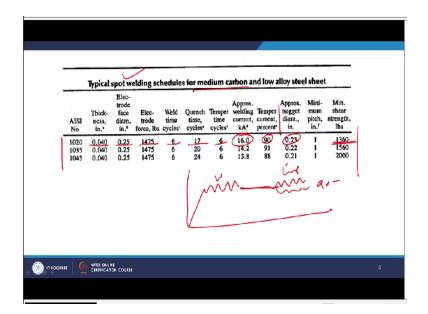
As compared to the low carbon steel if we see and medium carbon is as compared to the low carbon steels for a spot welding and the seam welding. If we see spot welding of the medium carbon steel for these 4 types of the medium carbon steels and the mild steel like 1020 for 0.04 inch. The electrode phase diameter is the 0.25 electrode force is much higher like 1475 lbs weld cycle time is 6 cycles.
