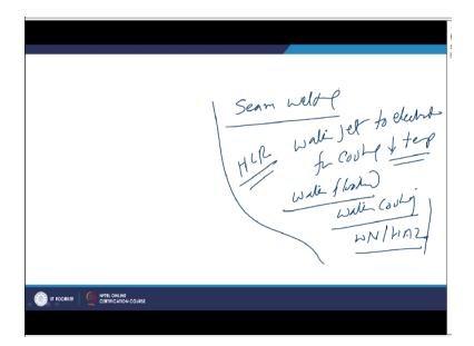
And there is another aspect related with this like in some of the welding resistance welding processes like seam welding it may be required to apply the water jet to the electrodes for cooling the electrodes, so that the electrode temperature is maintained within the safe limit. And in this process because of the water is a flooded there due to the cooling of the electrodes.
