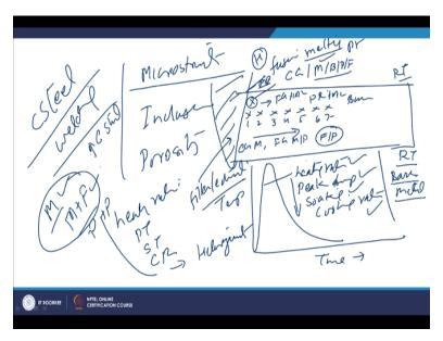
Now we will see that the way by which carbon steels behave, so ah this behaviour of the carbon steel during the welding will be observed in number of ways one is the way by which microstructural variation which is observed and the second one is the way by which the inclusions present in the steel will be responding and then third is the kind of the pores which are formed during the welding of the carbon steel.
