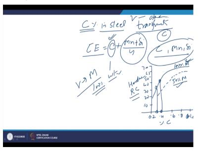
And there is a direct since the carbon steel since the carbon content carbon percentage in steel directly affects the tendency for the transformation or the transformation characteristics of the austenite to the other phase transformation characteristic is directly fitted by the carbon content and the alloying elements having the effects similar to that of the carbon content is taking care of to the carbon equivalent.
