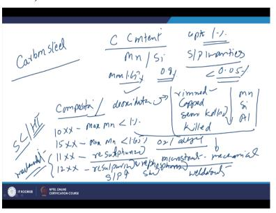
So will have to see this what are the various category of the carbon steels. Carbon steel means where primarily the carbon content is controlled and the carbon content can vary from like say up to 1% while there will be the residual elements like manganese and silicon as per the type of steel sulphur and phosphorus are there as impurities, sometimes their concentration is intentionally increased.
