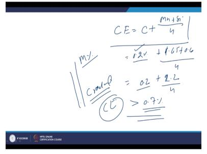
There is another aspect as I have said the carbon steel carbon equivalent is very important consideration in welding of the carbon steels which is calculated using carbon+manganese+silicone/4. So this will give us the carbon equivalent, so if we take and
