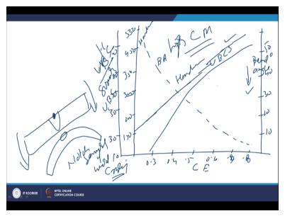
But it will in if the section thickness is are high then it will further increase the tendency for the cracking. So there is very useful diagram which is showing the relationship between the carbon equivalent and the various other properties in form of like one side we have the bend angle a well is made like this, then notch is made in the weld phase side and then controlled bend test is carried out to see the extent of twitch bending of the weld joint can be done.
