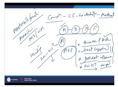
The martensitic transformation is directly linked with the composition of the steel, if the steel is of the high carbon equivalent it will show the higher hardenability and which will show the increase the tendency for the martensite formation. So the steel if the steel microstructure of the steel being formed either in the heat affected zone or in the weld metal if it is having the martensite or bainide or pearlite or ferrite.
