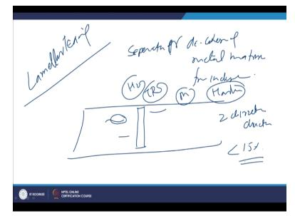
Lamellar tearing is basically about the separation or decohesion of the metal matrix from inclusions so like a steel having the inclusions like this, so these inclusions get separated from the matrix about it is promoted by the presence of the hydrogen tensile residual stresses hard martensitic structure, high hardness as well as the Z direction ductility. This is basically the ductility of the metal in the thickness direction.
