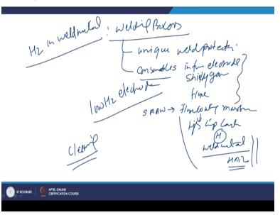
And that requires extreme care to facilitate the welding, so as far as the hydrogen induced cracking is concerned they are 3 important aspects to be present for which will facilitate the occurrence of the hydrogen induced cracking these include like the favourable microstructure and which is basically the presence of either martensite only or the presence of martensite and the ferrite in the matrix of the steel.
