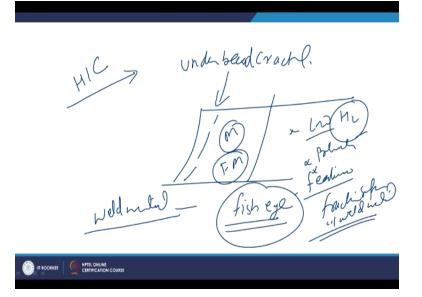
And that intern will help in reducing the hydrogen induced cracking tendency, then we have the most common form in which the hydrogen induced cracking observed is the under bead cracking. Under bead cracking is mostly observed in next to the fusion boundary in the base metal, so the cracking which is occurring next to the fusion boundary in the heat affected zone is mostly considered as under bread cracking been triggered by the hydrogen induced cracking.
