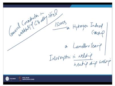
So we are starting our this chapter this presentation with the weldability of the carbon and low alloy steel. So it basically includes the general considerations related with the weldability general considerations in weldability of carbon and alloy steel or consideration visually includes the kind of the issues which are experienced in the welding of the carbon and alloy steels.
