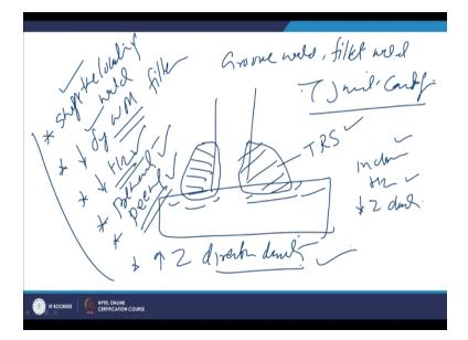
Like say joint is typically like this so the development of the weld this manner will be setting up of the higher residual stresses in the weld zone, so due to the shrinkage the setting of the tensile residual stresses will be setting up the metal next to the weld zone under the very restraint conditions and if there is a presence of inclusions as well as hydrogen and so the high tensile residual stresses inclusion, hydrogen as well as the limited Z direction ductility.
