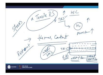
Then the stress is the another important aspect that has to be there to facilitate the hydrogen induced cracking and other the these stresses are if these are of the tensile in nature, tensile residual stresses, then it will be promoting the hydrogen induced cracking tendency significantly. So all those steps methods which can be applied in order to reduce the magnitude of the tensile residual stresses that will help in reducing the hydrogen induced cracking tendency.
