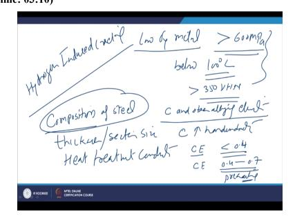
So we will start with the hydrogen induced cracking normally the hydrogen induced cracking is not observed in case of the low yield strength metals or low in strength steel. So the yield strength of the steel is greater than roughly 600 MPA, then the steels become sensitive for hydrogen induced cracking and especially it occurs at temperature below 100 degree centigrade.
