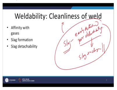
Some types of the slags which are formed during the welding they can be easily detached but there are few types which show the detachability and when the flag is not detect properly from the weld will then it may remain attached and that can lead to the formation of the slag inclusion. So the slag detachability and amount of the flag which is being formed both affect the cleanliness of the weld metal.
