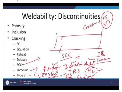
Cracking of the weld joint of the steel is also observed and in the corrosive environment when we either apply the external tensile stresses or the residual tensile stresses developed in the matter. So the metals which are sensitive to the corrosion as well as they are experiencing the tensile stresses or the tensile residual stresses. This show increased cracking tendency along the
