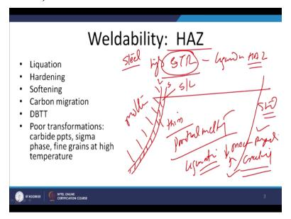
As far as heat affected zone is concerned even in case of the steels which are having the higher solidification temperature range, they show the liquation in the region next to the fusion boundary like this if the we know that if the steel is welded any zone which is heated above the liquidous temperature will be brought to the molten state. But there after there will be a zone which will be (()) (07:14) and that will falling in the solid liquid region.
