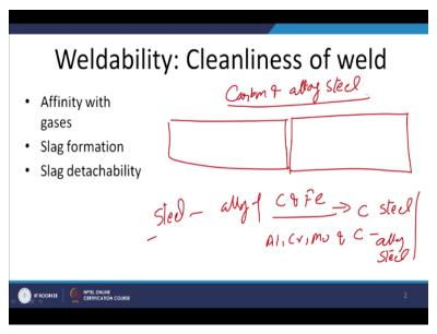
So like say especially with regard to the steel welding no steels is an alloy of carbon and iron. So when only the carbon content is controlled it is called carbon steel, but when other alloying elements like aluminium, chromium, molybdenum is also added in control way apart from the carbon then it is called alloy steel. So in this topic basically will be initially talking about the weldability of the carbon and carbon steel and alloy steels.
