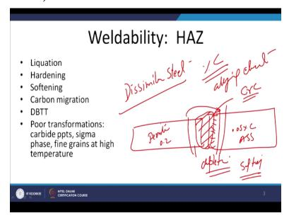
In that case like one side we are having the very low carbon steel the system like 0.05% carbon in austenitic stainless steel and on the other hand we are having simply ferritic steels having like say 0.2% carbon. So whenever these are the fusion welded what will notice that there is a movement of carbon from the high carbon zone to the low carbon zone due to the concentration gradient.
