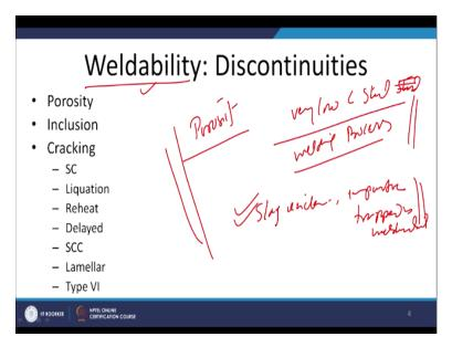
as far as the discontinuity development is concerned in the steel weld joints of the common the discontinuities which are observed in the steel weld joints and dictate the weldability of the steel is the porosity. Porosity is primarily observed in case of very low carbon steels and those when the welding process is not well controlled.
