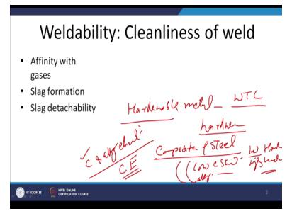
Since both are of the hardenable metal systems means the hardenability means hardenable metals which means when whenever they experience the weld thermal cycle they show such kind of metallurgical transformations where increase in hardness of the metal takes place. So however the hardenability of the metal will depend upon the composition of the steel low carbon steels or of the low hardenability while high carbon steels are of the high hardenability.
