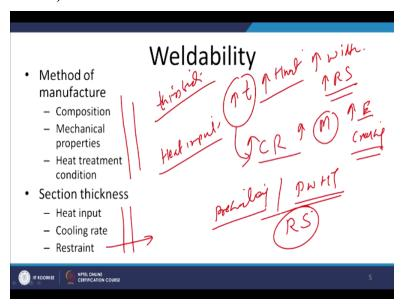
But when we talk of the weldability of steels for thick sections we need to consider the additional aspects like heat input like a greater is the section thickness greater will be the net heat input requirement, greater will be the width of the Hz and greater will be the residual stresses. So there will be lot of issues related with the greater heat input when the heaver sections are welded for the section thickness is more it will be extracting the heat more rapidly from the weld metal.
