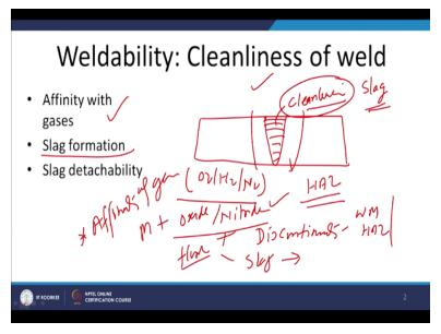
So most of the steels show the carbon and alloy steel show the hardenability and that is why there are 2 important aspects that are looked into to see the weldability of the steel, one is the of the cleanliness of the weld metal which is all about the slag kind of the slag which is present in the weld metal or if it is free from the slag and another one is the kind of the heat affected zone property valuation.
