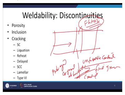
So a fine grain zone is formed fined grained Hz zone is formed as well as in this region on the prolonged exposure at high temperature formation of the unfavourable carbides at the grain bound at the grain boundaries of the fine grain leads to the promotes the cracking in the region away from the fusion boundary wherever fine grain zone, fine grained heat affected zone is present.
