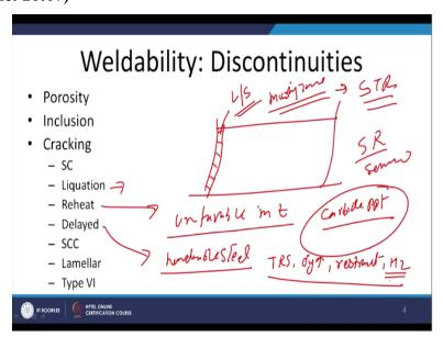
Then the liquation cracking is observed in the region next to the fusion boundary wherever the 2 phase zone is found both solidus as well as both solid and liquid phase are present and this is the basically the (()) (20:25) will be wider in case of the alloys having the wider solidification
