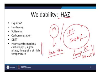
So formation of such unfavourable phases and intermetallic compounds in the heat affected zone sometimes leads to the reduced performance of the weld joint and reduced ductility, reduce the weldability of the metal due to the unfavourable metallurgical transformations. Apart from these phase transformations there can be formation of the martensite site.
