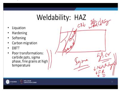
Then there is like as per the heat affected zone is concern many unfavourable phase transformations in the heat affected zone can take place in the steel and one of them is like in the steels like stainless steel specially the formation of the chromium carbide at the grain boundaries, this kind of the chromium carbide formation lowers the corrosion resistance and this is also called weld decay .
