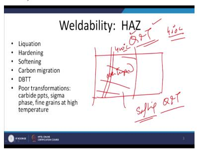
So obviously it is properties will be corresponding to the quenching and tempering for a corresponding to particular temperature saying steel has been quench and tempered at 400 degree centigrade. So during welding the heat affected zone will be formed and any region which is heated above 400 degree centigrade that will be over tempered and we know that over tampering invariably leads to the softening.
