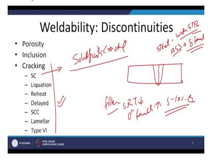
The steel weld joint show various types of the cracking tendencies like the first one is the solidification cracking. Solidification cracking is typically observed in the weld centre line at the weld centre line in the steels which show the wider solidification temperature range in austenitic stainless steel it is observed when the delta ferrite is very limited. So the weld centre line immediately after the building will show the cracks in the weld joint.
