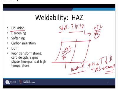
Whenever steels which commonly only have the pearlite, ferrite, bernide in the phases which are completely soft phases when they are subjected to the unfavourable weld thermal cycler these lead to the formation of the martensite and the formation of the martensite in the heat affected
