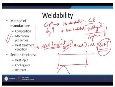
Now we will see that the factors as far as the steel circumstance the factors that affect the weldability like the most important factors that are affecting the weldability of the steel is like composition because it directly affect the hardenability due to the change in the carbon equivalent. Then the mechanical properties in general it is more difficult to weld the metals of the high yield strength.
