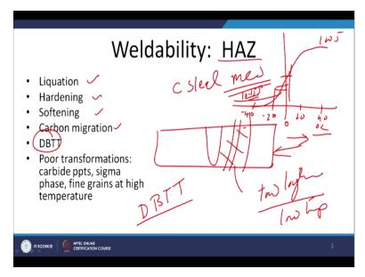
And which in turn reduces the corrosion resistance and sometimes hardening of the steel is also caused due to the localized carbon enrichment apart from these undesirable effects like liquation, hardening, softening, carbon migration. There is another undesirable feature or unexpected behaviour which is shown by the heat affected zone steels in the heat affected zone is the in case of the carbon steels like a medium carbon steel when they are subjected to the welding.
