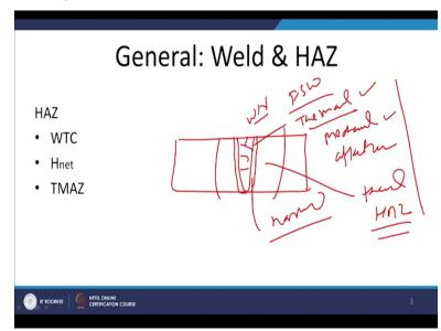
So the zone which is completely deformed fractured refined is called weld (()) (25:28) in case of the FSW while the zone next to the (()) (25:34) is the zone which experiences both effect of heat and effect of the deformation. So that is why it is called thermo mechanically affected zone. This zone is very narrow and thereafter region is formed which is affected only by the heat being transferred from the (()) (25:57) to the base metal.
