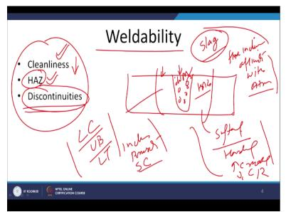
Since the weldability of the metals considers the properties of the weld metal as well as the heat affected zone. So we need to consider the 3 aspects whether the weld metal is clean or not, clean means it is free from the slag or the flux inclusions or not that will depend upon the kind of the
