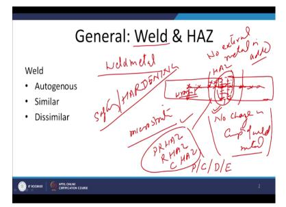
So if we talk in the begging about the weld metal the weldability when we are looking in weldability of metal when we are looking into the weld metal related aspects. So a weld joint of a given metal can b e produced just say either by fusing the faying surfaces and so the metallurgical continuity is realized after of solidification. In this case no external metal is added this in this case there is no almost no change in composition of weld metal.
