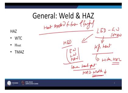
As as I have said we have the option to regulate or adjust the composition as well as the weld metal properties by choosing either the matching filler metal or of the completely different kind of filler metal. So that the weldability related issues of the base metal can be reduced. But we cannot do much as far as the heat affected zone development is concerned, because it is directly affected by the amount of heat being supplied for fusion of faying surfaces.
