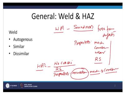
Because soundness whether it is free from defects and discontinuities or not and if it is free then what are it is properties in terms of like mechanical properties, corrosion properties, wear properties or then what are the kind of the residual stress development in the weld metal and accordingly will be saying whether the weldability of metal from the weld metal point of view is good or **or** it is poor .
