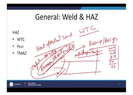
So the heat affected zone so sometimes we get the thermomechanically affected zone apart from the heat affected zone also. so now we know that heat affected zone which experiences various weld thermal cycles as per the metal system it may experience the recovery and recrystallization in case of the work hardening metals grain refined metals, dispersion harden metals, even transformation harden metals.
