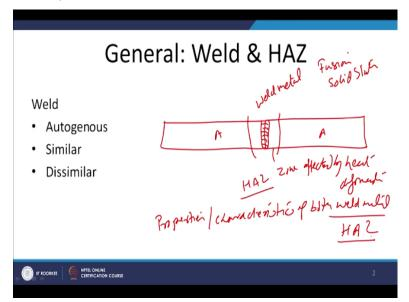
How the weld metal properties and the heat affected zone properties are affected. So like the metal, the 2 parts of metal A are being joined either by the fusion welding or the solid state joining process, a joint will be produced at the interface in case of fusion welding it is typically
