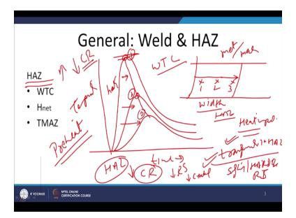
So heat affected zone issues cannot be eliminated but certainly they can be reduced and it to a great extent means the Hz characteristics to a great extent depends upon the kind of well thermal cycle being experienced by the base metal in the heat affected zone, like heat affected it is the zone or the width up to which the base metal properties are being affected metallurgical and the mechanically.
