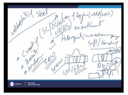
Now we will see what kind of the basically in the weldability of the metals we have to talk at length about the weldability of the ferrous systems. So, which primarily comprises the weldability of steels. So, the steels during the welding primarily suffer from the loss of toughness of the weld as well as heat affected zone, this is called embrittlement, so their ability to sustain the impact loads is reduced drastically.
