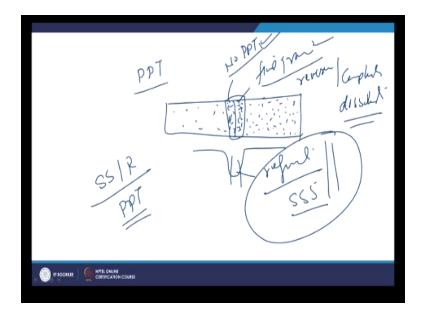
On the other hand if it is the precipitation hardenable aluminium alloy which gets it is strength from the formation of fine precipitates. So, controlled plastic deformation of the weld metal near the faying surfaces will be leading to the very fine grain structure. But the fracturing and the control plastic deformation followed by the high heat generation leads to the reversion and complete dissolution of the precipitates.
