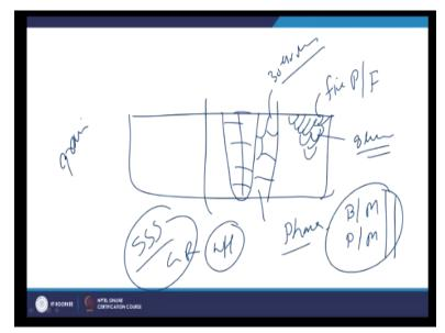
Like in a steel like say the steel the base metal is having very fine grain structure in form of fine pearlite and the ferrite. Average grain size is say 8 micro meter and due to the welding like say either fusion welding or the deformation based process heat generated leading to the coarse grain structure in the heat affected zone. So, this coarse grain structure maybe leading to the very coarse grains in the heat affected zone and say like 30 to 40 micrometer.
