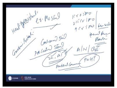
Next category of the steel is the heat resistant steels these are basically chromium molybdenum steels there are various chromium molybdenum like 1 chromium, 0.5 molybdenum 2.25 chromium, 1 molybdenum. Then 9 chromium, 1 molybdenum, so there are various combinations of the chromium molybdenum steels which are used for the high temperature applications like 600 to 650 degree centigrade in thermal power plants.
