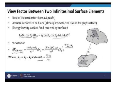
So how do we evaluate this view factor mathematically? So view factors basically gives you an idea how much rate of heat transfer activity place between surface  $A_i$  or first surface and surface  $A_j$  the second surface. So although the definition of view factor is equally applicable when the surfaces are gray. That means their emittance and absorptance does not depend on wavelength.
