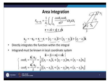
So we have the first method, the first analytical method is the area integration where we have to basically integrate over the surfaces to evaluate the view factor.
