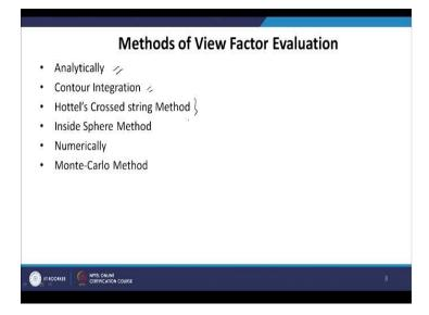
We can do double integration that is called analytical method. There are simplified methods like contour integration which basically simplifies the double integration, double surface integral into line integral, the path integral. Then, we have Hottel cross string method, inside sphere method. We can use numerical methods where we divide the surface into a small number of infinitesimal surfaces.
