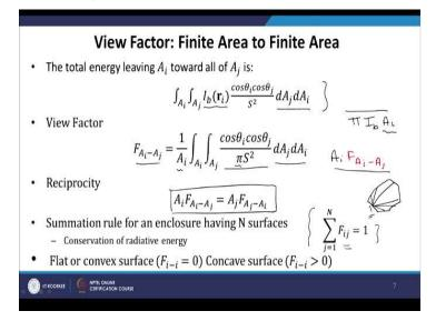
Now in the case where we calculated view factor between infinitesimal areas, we just integrated over area  $dA_j$ . Now when we are trying to find out view factors between two finite areas, we have to do double integration and this double integration has to be taken place over the entire surface  $A_i$  and surface  $A_j$ . So the total energy emitted from surface  $A_i$  is  $I_b cos \theta_i dA_i$  and this surface energy basically reaches the surface  $A_j$  okay.
