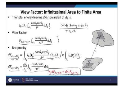
So if we want to find out the surface area or this view factor that is view factor from a small infinitesimal surface  $dA_i$  with whole surface  $A_j$  we have to basically extend the same logic, the total energy leaving surface  $dA_i$  towards the entire area  $A_j$ . So all we have to do is use this previous expression that we basically used. We used this expression  $I_b dA_i \cos \theta_i d\Omega_{ij}$  and just multiply or integrate over the entire area  $dA_j$ .
