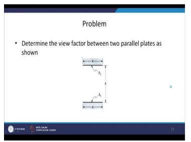
So let us conclude this chapter with one example. So we have two parallel plates, the width of each plate is w and the distance between the vertical distance or the separation between the two plates is h and the plates extend to infinity that means the thickness of these plates in the plane of the board or paper is infinity. So we have to evaluate the view factor for this configuration. (Refer Slide Time: 25:47)
