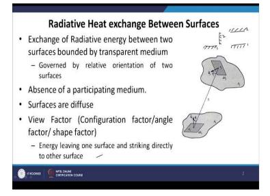
So it is pretty much very much clear that amount of energy exchanged from one surface to another will depend on orientation of the two surfaces. So for example, we have two surfaces having the same area and similar temperatures. If their orientation is not same, the amount of energy transferred from one surface to the other will not be same.
