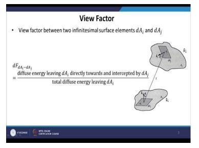
So the definition of view factors goes like this. For two surfaces,  $A_i$  and  $A_j$  let us consider some infinitesimal areas  $dA_i$  on surface  $A_i$  and  $dA_j$  on surface  $A_j$ . Thus, view factor between these two infinitesimal surfaces is defined as
