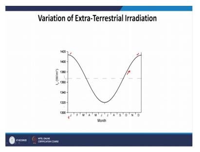
Now, we see that, how the solar radiation basically reaches earth. On top of the earth's atmosphere. So, basically when we look at this radiation coming from sun, the radiation from the sun, we assume that the sun behaves like a black body. The temperature of the sun is around 5700 kelvin, 5700 to 5800 kelvin. That is the temperature of the sun surface. And at that temperature sun behaves just like a black body.
