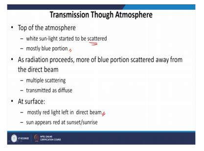
Now, how the transmission of solar radiation is basically being affected? So, let us look at a closer view of that. So, radiation reaches on top of the atmosphere, the intensity is not affected. The intensity is same as it was at the surface of the sun. Now, once it starts entering the earth's atmosphere, it undergoes scattering. On top of the atmosphere, intensity is not affected. But as it enters the atmosphere, it undergoes scattering.
