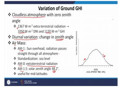
Now, how these clouds, these gases and aerosols affect solar radiation at the ground. So, we just take extraterrestrial radiation is 1367 watt per meter square. We discussed this in the previous slide. So, around 1367 watt per meter square is the extraterrestrial radiation reaching outer atmosphere. And when it penetrates through earth atmosphere, there may be cloud there may not be cloud.
