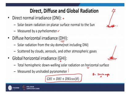
So, we have sun and we have a surface. So, there is a direct component. This direct component definitely change with the inclination of sun. It depends on zenith angle. And then, there is a diffuse component. Basically, radiation coming from all the direction, that is diffuse. There is not much effect of diffuse radiation by the zenith angle. So, direct solar radiation, direct normal irradiance is called basically the beam radiation.
