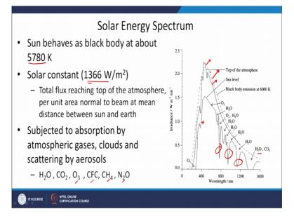
Now, how the spectrum looks like, how the variation looks like when this same radiation enters the atmosphere. And this figure of irradiation at any point on the surface of the earth, we have seen it earlier also. So, we have 3 different curves here. 1 is basically the black body intensity. The second one is extraterrestrial radiation. And third one is basically the terrestrial radiation, that is radiation received at the earth surface.
