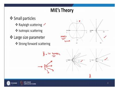
It is represented by the scattering phase function which is = 1 for isotropic scattering. If the scattering is isotropic, the scattering phase function is 1. Now, scattering phase function can also be derived from the Lorentz Mie theory using Maxwell's equation. Same theory can be used to find out the scattering phase function. We are not going into the details, the mathematical details.
