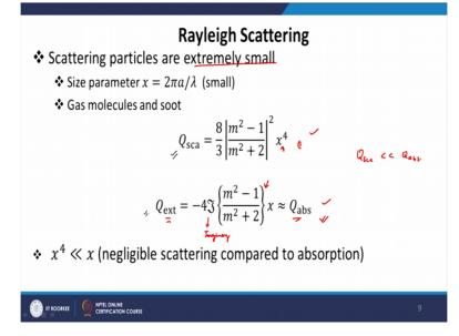
We can simplify the mathematical relation. And the scattering efficiency and extinction efficiency is given by these relations. So, we have scattering efficiency is = 8 by 3 m square – 1 upon m square + 2 whole square x power 4, x is a size parameter. And we have extinction efficiency which is = -4, imaginary part. This is imaginary part of m square – 1 upon m square + 2 into x, which is now = just absorption efficiency, because the this term is much larger than this term.
