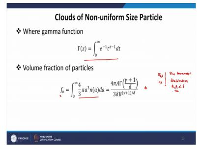
So, the gamma function is given by this relation. This is the gamma function. So, if we assume that a particle size follow modified gamma distribution, we get the total number of particles. We also define 1 more parameter for particle cloud, what we called volume fraction of particles, that is the total amount of space occupied by the particles. So, volume fraction is defined as volume of single particles, 4 by 3 pi a cube.
