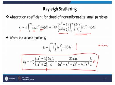
Kappa lambda is = absorption efficiency factor. Then multiplied by the size distribution. And we take modified gamma function as the size distribution. And this comes out to be -4 imaginary part of m square -1 m square +2. And then, this size distribution function. So, I am just leaving this as an exercise to derive from this here. Now, this time in the bracket is called volume fraction.
