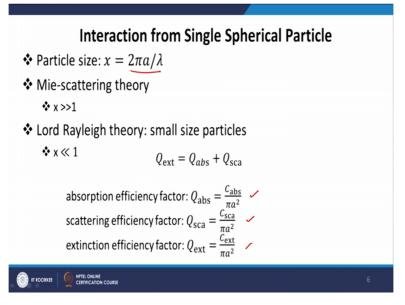
So, to decide what type of scattering will take place, we have to first look at the size parameter. The size parameter is defined as; assuming that all the particles that we have are spherical in nature. So, this is just a size parameter defined by assuming that the particles are spherical in nature with radius a. So, we define a particle size parameter as 2 pi a by lambda, where a is the radius of the particle, spherical particle.
