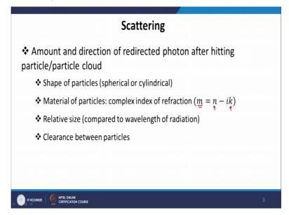
So, how this scattering is basically depend on the properties of the particles, how scattering depends on what kind of particles we have, it can be basically broadly understand understood based on 3 major parameters. The first one is, what is the shape of the particles. If we have spherical or cylindrical particles, of course in real life the particles may not be actually spherical or cylindrical, they may have arbitrary shape.
