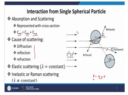
So, scattering is basically a phenomenon which is governed by 3 physical processes, the reflection, the refraction and diffraction. So, we have 3 physical phenomena basically that govern the process of scattering. And as you see here, reflection is basically a phenomena where light strikes a particle and it bounces back and it travels in a different direction. This is reflection.
