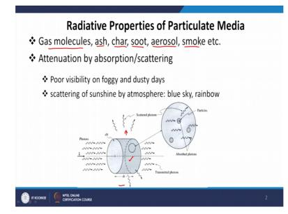
So, we understand that the particles, they tend to absorb and scatter radiation. As is clear from this image, we have bunch of photons coming. And when they enter the medium which is having particles that absorb and scatter radiation, some of the photons are attenuated or absorbed within the medium. And some of the photons are scattered in this direction. In fact, that scattering may actually depend on direction.
