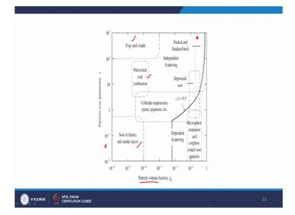
Now, we have a different type of applications, where we have different type of clouds. We have fog and cloud. We have also have pulverized coal application, soot. Okay. So, depending on application, we have different volume fraction for this particles. For example, the soot in typical flames and smokes has very small volume fraction and the particle size is also very small. Okay.
