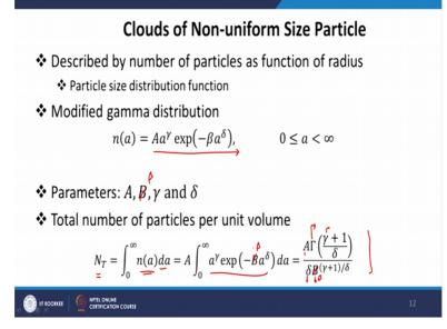
Modified gamma distribution, with parameters A, beta, gamma and delta. So, this is a distribution that is basically followed by the particles. This is beta here. So, we have what we called modified gamma distribution, generally defining the size distribution of the particles. What we do now is, total number of particles is basically = number of particles of size a all the particles here also are assumed spherical in shape.
