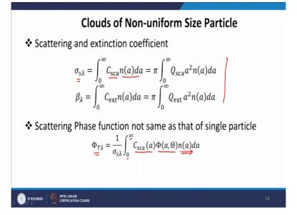
So, expression for scattering coefficient is, scattering cross-section multiplied by that number of particles of a given size. And when we integrate it, we have to basically find out this scattering coefficient and absorption coefficient in terms of the size parameter A, beta, gamma and delta. So, we will solve this equation for 1 example. But ultimately, the solution comes out to be in closed form, in the form of gamma function.
