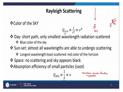
Now, looking at this relation, so from heat transfer point of view, the scattering efficiency factor is not important. But just for the sake of scattering from atmospheric physics point of view, we understand that the scattering efficiency is proportional to 1 upon lambda power 4 or frequency power 4. We have x power 4 and x depends on 1 upon lambda. So, the scattering efficiency factor is proportional to 1 upon lambda power 4.
