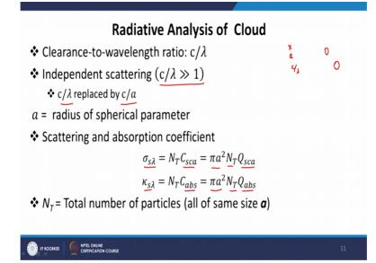
So, so far, we basically found out Rayleigh and Mie scattering for individual spherical particles. The same theory we can extend to a particle cloud. Now, particle cloud basically have 1 more additional parameter. So, the 2 parameters are size parameter x, as we discussed. And we also discussed the particle diameter a, if they are spherical in shape. Now, we have to talk about what we call clearance to wavelength ratio c by lambda.
