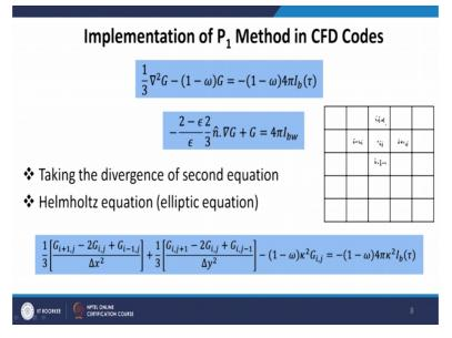
Now, how to implement this method in safety codes. So, as engineers, we all know how to program or discretize the partial differential equations. This is elliptic type of partial differential equation. We call it Helmholtz equation. We can discretize this on any domain. I have taken this here. A cartesian system on in a 2-dimensional domain, cartesian mesh, you can discretize it using central differencing scheme.
