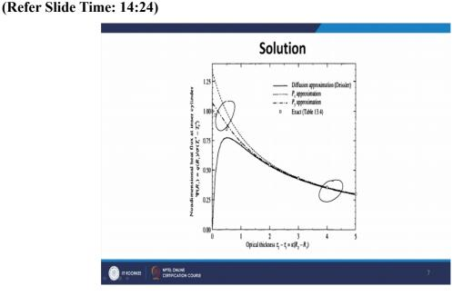
What you see here is a, the non-dimensional heat flux at the inner cylinder versus optically, optical thickness. And you see that under optically thick condition, the P 1 method, P 3
