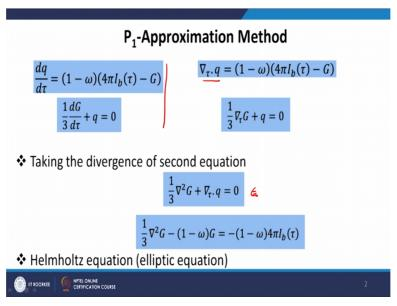
The first equation is dq by d tau is = 1 - omega 4 pi I b - G. This is the first equation. And second equation is, 1 by 3 dG by d tau + q. So, these equation, we derived in the framework of 1-dimensional plane parallel slab. But they are general, because the only assumptions while driving these equations was that the intensity does not vary with azimuthal angle. And we took first 2 terms of the spherical harmonics in deriving those equations.
