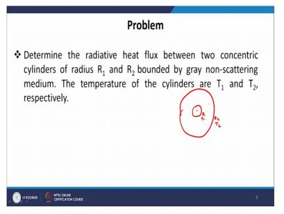
The medium inside the cylinder is gray and non-scattering. So, we have to find out the heat flux between the 2 cylinders. So, we have cylinder 1; second cylinder; this is the center. This cylinder is radius R 1 and temperature is T 1. And this is R 2 temperature is T 2. We have to find out how much heat flux is basically happening between these 2 cylinders. So, let us solve this problem.
