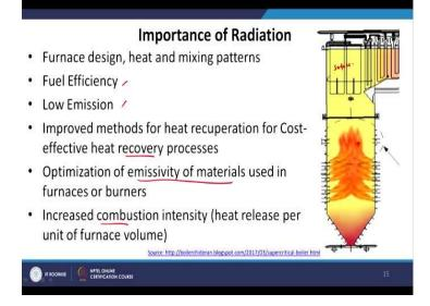
Now why we are studying radiation because there are many things that we want to optimize. For example, in this furnace in the furnace we burn coal and due to burning of coal we have flue gases forming, these are the flame and this flame basically carry heat or through convection but also significant amount of radiation is there and this radiation reaches the surfaces in the top part. These are the heat transfer surfaces of the boiler.
