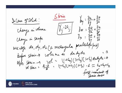
Now, in the case of strain what we see is that what we got the shear strain as gamma x y then gamma y z and gamma x z. So, since you have the 3 components of the shear strain and this is as we know that this is dou u by dou y plus dou v by dou x.
