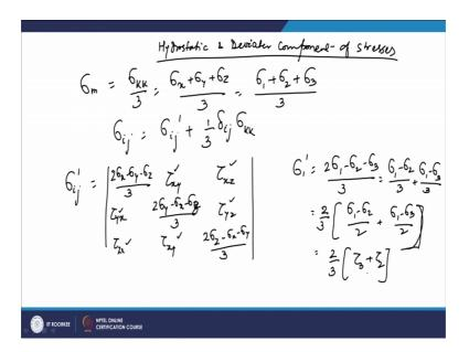
Now, so you have hydrostatic and deviator component of stresses. So, now again as we discussed that, in the case of strain, we found. Similarly in the case of stress also you have the 2 components; one stress will be required one stress, which is responsible for the change in the volume that is known as the you know hydrostatic stress or the mean stress and the stress component which is responsible for the change in the shape that is known as the deviator component of the stress.
