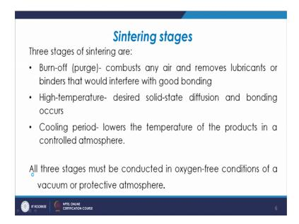
So, as we discussed that these three stages which are defined in case of a sintering. They are first stage is the Burn-off stage that is purge stage. Now, in this burn-off stage, when you are increasing the temperature in that case whatever gases are there inside in air or any lubricant which is there inside the green compact.
