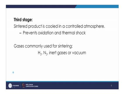
And it will be preventing the oxidation and thermal shock and the gases which are normally used for sintering is the hydrogen nitrogen inert gas or vacuum. So, basically you are doing that in a controlled atmosphere in the presence of the such you know inert gases in which the third stage three stages of the sintering is carried out.
