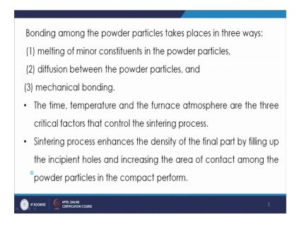
So, basically there are three stages in which the basically the bonding is developed. First is in the first stage you have melting of minor constituents in the powder particles. So, what happens that if you have minor constituents have lower melting point materials they are melted, if you have volatile substance is they are driven off. So, that happens in the first stage. Then what happens that you go to the second stage and in the second stage you have a diffusion between the powder particles.
