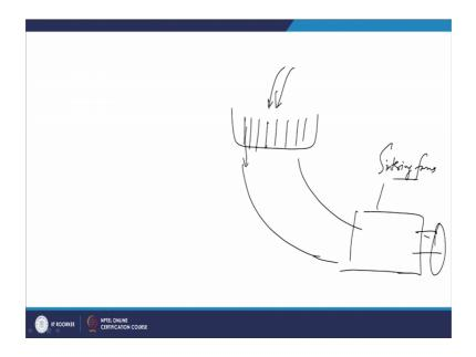
So, the powders will be there a in; so, powders will be coming and then once they are coming. So, there will be following through a route and then basically there is a furnace. So, there will be a sintering furnace. So, this sintering furnace is used so once there will come and in form of a sheet and then that is further you know under the application of a rollers, there will be further rolls that way you can get a rolled you know sheet even in the case of by using these powders.
