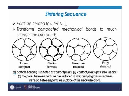
So, parts are normally heated to about 0.7 to 0.9 times the melting temperature of the material normally that is in the form of kelvin and then, so that way the compacted mechanical bonds to this you know much stronger metallic bonds you know they are converted to.
