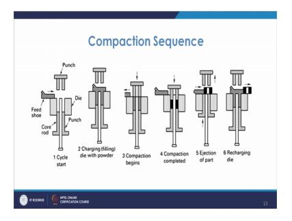
You see that you have the start of the cycle where you have this is the die and in that basically you have. So, this is a cavity in which this material is kept as a powder is kept and then from the top you will have the punch the top part will come and it will apply the pressure; so a dimension or height of this much.
