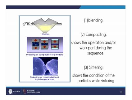
So, this process talks about the blending then once you do the blending; then you are going to compact its. So, compacting you apply this pressure and you; so, I will compacting you can see that the space between then is there that is decreasing and that is further decreasing.
