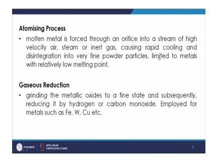
So, in that atomising process basically you have a the spray of the material atomized form.
