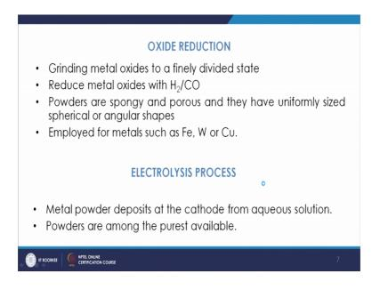
So, the we are discussing about the oxide reduction; so oxide reduction is normally you have the use of hydrogen or carbon monoxide ad we use that. So, that we are already studied you have you know deposition at the cathode and they are very pure.
