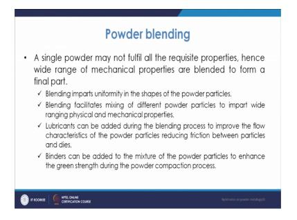
So, this is how you know we go. So, what happens that it normally in a you have a you know ball mill. So, you have a very large type of you know vessels in that you have these balls are you know refractory balls. So, hard balls steel balls or caped and they basically this is rotated. So, this will be basically rotated and then metal will be there inside and that basically comes under the impact you know of these balls that gets converted to the powders.
