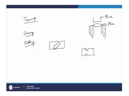
So, as we know that you know trimming is required for the force products where you have the flash found in the part in plane. So this flashes to be removed and in that case this flash are removed by the trimming operations, so in that case suppose you have force product.
