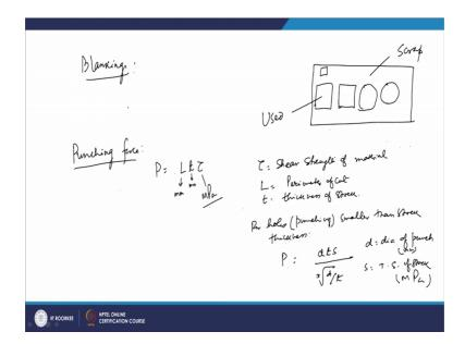
Now, in the case of blanking suppose you a sheet and in that basically you have to have a blank of certain sheet or you have a blank of certain shape, so basically when you use the punch this size of the blank is being cut and they are removed from the sheet. So then once you take such kind of you know blank from the different parts and then there may be you know all that so this part which is to be used and this part is the scrap.
