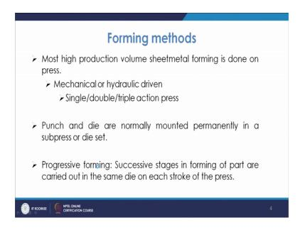
So that way you have progressive forming mostly when we go for the punching or sharing operations, so that comes under this kind of operations so that is under the progressive forming. So when the sample of the progressive forming as we discussed is this piercing and you have the blanking operations as we see, so this is a kind of punch which will be coming and it will be this is die basically.
