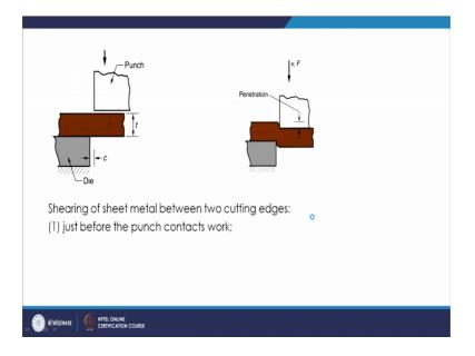
So, at this place there will be deformation at this way, at this place there will be you know so there will be trying to deform and ultimately you will have a penetration here and then ultimately the material fails and then it will be cut. So basically you have this given as the clearance and the fracture occurs you know in this zone, in this zone the fracture occurs and this will be shared slug.
