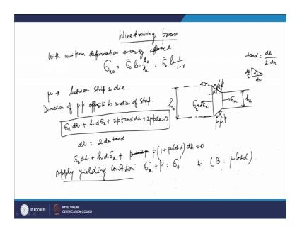
So, if you talk about the wire drawing operations. So, we will start with wire drawing process, now what we see is that if you use this uniform deformation energy approach; then normally with uniform deformation energy approach, we can get the you know draw stress values sigma x a and that will be basically average stress value and then l n of A b upon A a.
