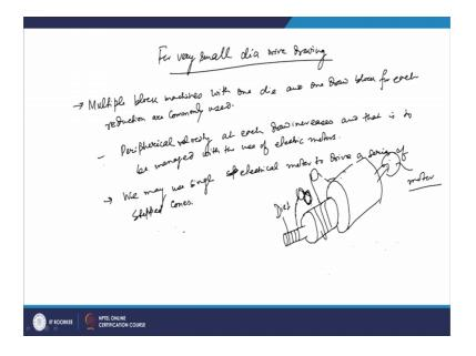
Now so, this is this will come later before that what we do is. So, in the case of these you know when we have to go for very small wire drawing, so you may use multiple you know block machines. So, multiple block machines with one die and one draw block for each reduction are commonly used.
