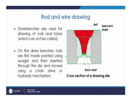
So, we will talk about the principle of the rod and wire drawing. So, what we do is normally such you know drawing dies there. So, this is the cross section of the drawing
