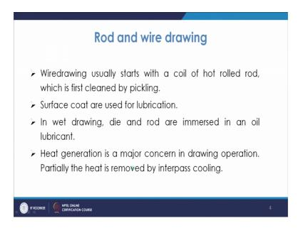
So, the pickling is done basically to ensure that there is no at all any kind of scale or dirt on the surface. So, that when you go into drawing the wires, then in that case that is a non-interfere with the drawing operation or if that is going into it that may result into certain kind of defects.
