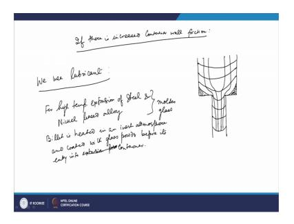
So, if there is increased container wall friction; now, what we see in the in such cases basically your you have distortion of this grid pattern takes place. So, in such cases, now in such cases what happens that when you have increased this friction between the container of wall and the billet.
