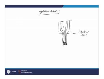
We will talk about extrusion defects. Now when we talk about extrusion as we know that when the metal is you know pressed from one side, the metal has to flow and there will be friction at the container, liner and the billet that interface the new friction and for you know decreasing that friction we apply the lubricants.
