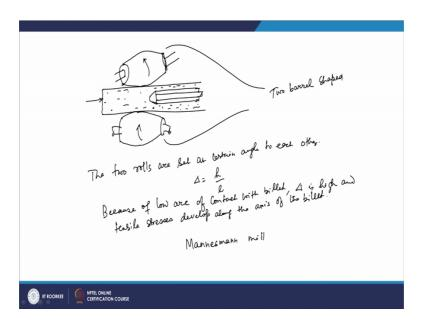
Now, in that case that have been done is suppose you have a billet which is there of suppose this thickness. Now in this case it has to be you know ah that tube to be extruded; now seamless pipe is to be extruded in the that case. Now this is used for normally the lottery piercing of the, you know steel and copper billets.
