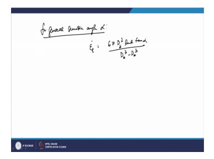
And if you lock c for the general semi die angle alpha so, for general semi die angle so, for general semi die angle alpha, if you try to calculate so, this epsilon t this will be 6 V Db square ln R tan alpha divided by Db cube minus De cube.
