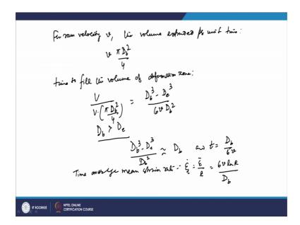
So, that will be the volume extruded per unit time. And if you see that time to fill, the volume of the deformation zone so, it is nothing but volume divided by they this area multiplied by this. So, you have you know so, area multiplied velocity so, this is a same thing. So, volume by volumetric you know expansion per unit time so, that will be the time. So, it will be V by V into pi Db square by 4. So, and that is has to be equal to Db cube minus De cube and divided by 6 V Db square.
