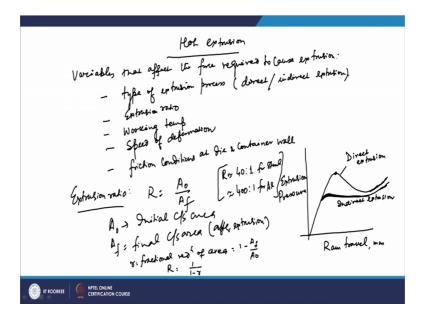
Now, there are many variables which have an influence on the force required to extrude the products. So, variables that affect the force required to cause extrusion. So, that will be first is type of a extrusion process. So, you may have the direct extrusion or you may have the indirect extrusion. Then you have the Extrusion ratio.
