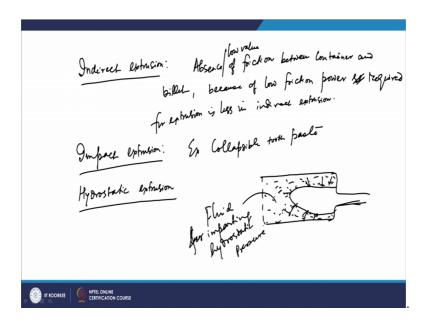
So, if you talk about indirect extrusion. So, the absence of friction between container and billet, because in this case the container along with billet that is basically pressed, there will not be any you know friction which is there.
