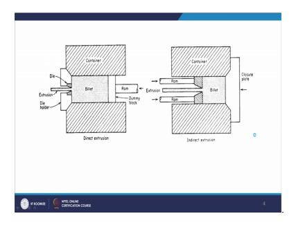
So, this is how we can understand the example of a direct extrusion and indirect extrusions; as we see that in this case you have a the direct extrusion, you have a die holder here and you are having the Ram here; you have a dummy block placed here.
