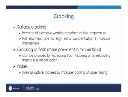
Now, the surface cracking is because of the excessive working of surface at low temperature and, also this hot shortness is due to the high sulfur concentration in the furnace atmosphere. So, that is what we see this these are the reasons, because of you know this the surface cracking takes place, cracking at the flash and this is more prevalent when the flash is thinner. So, normally you know the flash needs to be trimmed.
