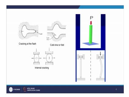
So, what we see here you can see that in this case, you have this is the flash and if this crack is there and this crack may be seen in the you know inside the casting itself.
