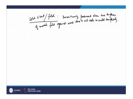
Now, this is the basically discontinuity which is produced, when the two surfaces of the metal are folding in each other and, they are not welding completely. So, this will be the discontinuity produced when two surfaces of metal fold against each other and, not able to weld completely.
