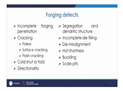
So, there may be reason for it may be thin may too thin flash or so, the severity is there in the case of flash cracking is that is a cracking is there in the flash and, if it has extended to the you know casting then the casting will be you know rejected.
