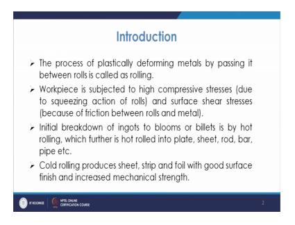
So, what we see is that the roll process of plastically deforming metals by passing it in between the rolls. So, that is known as rolling. Then Work piece is subjected to very high compressive stress due to the squeezing action of the rolls.
