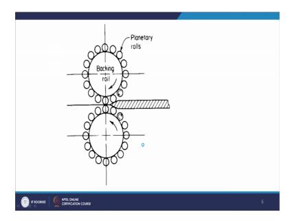
Then you have another kind of you know rolling, where we use these planetary rolls and this is known as the planetary rolling mill. So, this is planetary mill.
