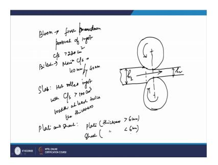
And what happens that these rolls; so, they will have this common center this is the center point and the. So, this will be rotating in the direction and this will be rotating in this direction.
