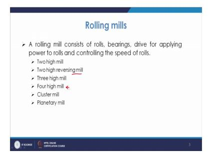
So, the rolling mill will become consisting of rolls, bearings, drives for applying power to rolls and controlling the speed of rolls. So, that is a way set up will be there. As we know that in the rolling mill you have you must have the means to rotate these rolls.
