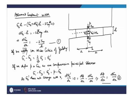
So, we have such is the strip and it has, the thickness is constant all along and it is in touch with basically the dies. So, these are the dies, on both the sides and now, in this basically, we are going to consider a strips. So, suppose you have a strip, which is of certain length. So, that these, this will be taken as of the length d x and we are applying the pressure.
