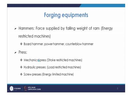
Now, in that board hammer or sometimes we also classify as the gravity drop hammer. And, then you have to drop hammer will be in fact, categorised as again for the gravity drop hammer and then you have the power drop hammer.
