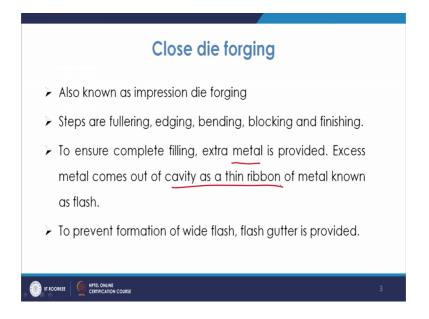
So, so that close die forging that is also known as the impression die forging because what happens in this case that you are ultimately trying to get the impression which is there into the dice. So, ultimate objective is to basically get that you know final shape of the material.
