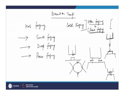
So, if we try to classify based on temperature then you have hot forging and cold forging.
