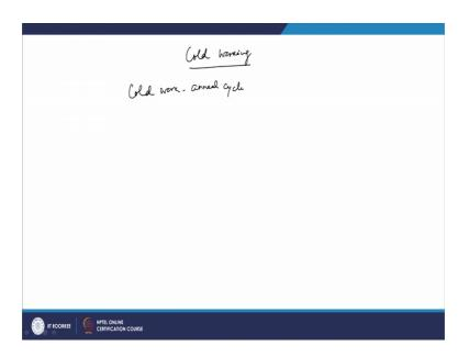
So, in the case of the strain hardening, basically material goes one getting harder and harder and your force as requirement as we have discussed that it goes on increasing. And in those cases you have the chances of cracking. So, what we normally do is, we are do the cold working stages you have a cold work anneal cycle.
