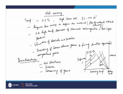
And, you know, in these cases the true stain values; which are achieved normally is quite high I mean it is it is there from 2 to 4 value is normally achieved. And normally hot forging or you have the hot extrusion or hot rolling is normally carried out, so that is what the advantage of the hot working is that you can go for the larger strain.
