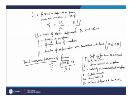
So, in those cases the maximum increase in the temperature. So, maximum increase in temperature so, that will be basically because of the work done on the material. So, that will be basically Td so, we call it as the temperature because of the deformation of the plastic deformation of the, you know, work piece. And so, this increase in temperature, and that will be divided by the, you know, specific heat of the material, and then you have the density of the work piece.
