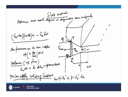
So, if you try to see that we try to analyze this slab method. So, this slab method it assumes that the metal is deforming; so, it assumes that metal deforms in deformation zone uniformly. The thing is the meaning is that if you have a square grid element, and if it is going under the application of stresses.
