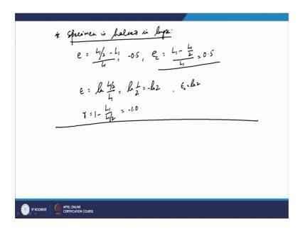
So, let us take for example, that if the specimen is halves in length. Now in this case, L 1 becomes L 1 by 2. So, we can find the engineering strain and engineering strain will be L 1 by 2 minus L 1 by basically L 1. So, it will be minus of 0.5, but if you take the engineering strain in compressive if direction compressive strain engineering compressive strain; in that case we will do the reverse L 1 minus L 1 by 2 and divided by L 1 so it will be basically 0.5.
