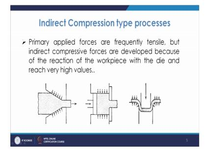
Now what will be happens in these cases like this is your tube drawing I mean this is wire drawing, so in the case of wire drawing what we see is you apply the force in this direction you are basically pulling. So, you are primarily you are taking the tensile type of primary primarily you are applying the force.
