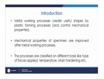
So, we have already you know studied about it that we use the plastic forming, we go the forming in the plastic state and then do the forming. So, mechanical property of the specimen are improved and certainly they are classified on different bases like type of forces applied temperature strain hardening etc.
