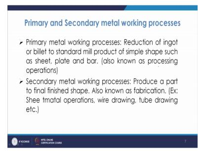
So, you are you have just like you do the rolling, forging or so intermediate one rolling basically. So those processes are where you are basically reducing the largest dimension of the product to the smaller dimension simple shapes than that is your primary metal working process and then when you are going for the final finished product, so they are known as secondary metal working processes.
