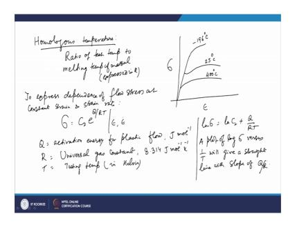
So, suppose you do it at minus of 196 degree centigrade; if the temperature is too low below the 0 rate centigrade temperature. If you go to minus of 196 degree centigrade you see that this is the stress strain diagram. Whereas, if you try to draw it at the room temperature something close to 25 degree centigrade then it looks like this so, it goes at about 25 degree centigrade. Whereas, if you further increase the temperature in those cases what you see is that this curve goes like this.
