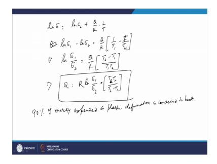
So, what we found is that 1 n of sigma will be 1 n of C 2 plus 1 Q by R into 1 by T. So, suppose you want to find the value of Q so, now, Q can be found. So, if you have sigma 1 at sigma 1 flow stress I mean if the flow stresses is sigma 1 at temperature T 1. So, log sigma 1 will be log 1 n sigma 1 will be 1 n C 2 plus Q by R into 1 by T 1 and similarly 1 n sigma 2 will be 1 n C 2 plus Q by R into 1 by T 2.
