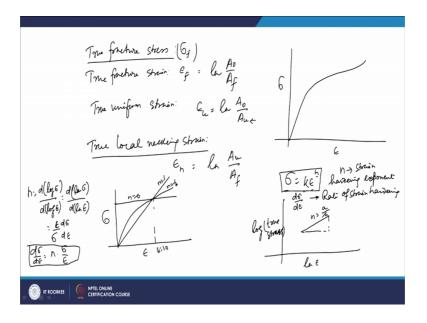
You must also know about the certain terms like you have the true fracture stress so, if you talk about those terminologies like true fracture stress. So, you go to the fracture point and at that time the true stress value which is calculated that is your true fracture stress and again that will be basically glowed at load which is there at the facture divided
