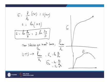
Now you can further try to refer to the, we can our we can recall our studies on the true stress true strain curve. So, as you see that when you have the true stress true strain curve so, you go to that and then this way it goes. So, this your true stress and true strain curve and here it fractures
