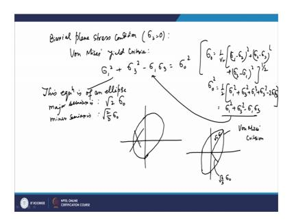
So, suppose we are talking about a biaxial plane stress condition. So, you have only sigma once a plane stress condition means you have only sigma 1, and sigma 3 sigma 2 1 of the stress 1 of the principal stress is 0 in that case and you have biaxial we are going to draw on the xy axis.
