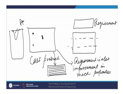
So, suppose you made one piece by casting of this dimension. So, this is your cast product. Now, you need a product of this type so, you need it. So, requirement is about this size of product. So, you can you can go for casting as we discussed that you can go for further the process of casting and, then you can make a smaller mould, you can have a smaller pattern and then you can make it.
