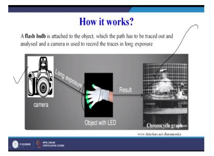
A flash bulb is attached to the object which the path has to be traced out and analyzed and a camera is used to record the traces in the long exposure and here you can see the white lines are there, these are the traces of the movement recorded by the camera and we have this light source attached to the fingers. So the LED light source is attached to the finger and this is recorded with the help of a camera.
