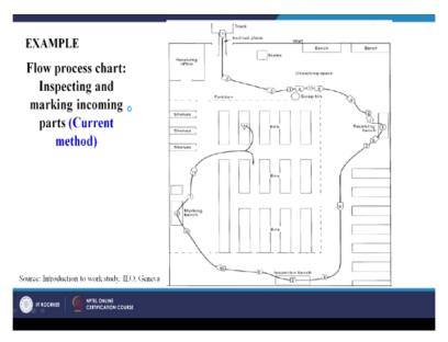
Now this is one example. You can see on your screen flow process chart inspecting and marking incoming parts. So what we are doing, we are inspecting and marking. So we have to do the inspection. So here you can see it is written very clearly truck. There is an inclined plane, all this information usually is missing in operation process chart, but in flow process chart it is given in a detailed manner.
