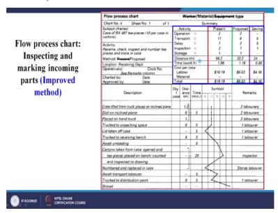
So if we see in the modified method the proposed method the distance travelled is 32.1 meter. Earlier in the present method it was 56.2 as we have seen here I have highlighted 56.2. So 56.2 has now been attacked and we have been able to reduce it to 32.2 by changing the layout of our shop floor. So all the other details you can look, but here we can see the number of transportations earlier in previous section were 11.
