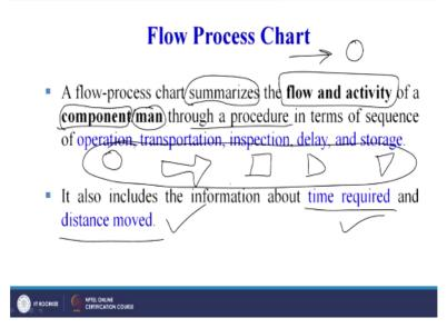
On your screen you can see that the flow process chart basically is the flow and activity of a component or men through a procedure in terms of sequence of operation, transportation, inspection, delay and storage. Once again, I will read it for you, you can see, flow-process chart summarizes, so the complete process is taking place, we will try to summarize that whole sequence of operations on a chart.
