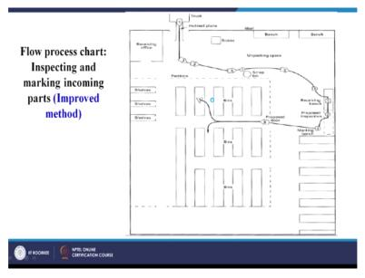
So we can improvise the method, it is coming from the truck, this method we cannot change but here you can see there is a receiving bench, inspection is happening, proposed inspection. So from our previous inspection which was happening somewhere here if we see in the previous slide. This is the inspection bench here. In the proposed one what we are doing. In the proposed one we are shifting it from here to here.
