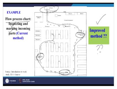
Now here you can see, this is one method of doing a work, it is a flow process chart of inspecting and marking the incoming parts. So here there is a truck from where the material is coming and this is the path being followed by the material before being stored in the bins, so there is a receiving bench here, there is a marking bench here and there is an inspection bench here, so inspection and marking are the 2 important works being done.
