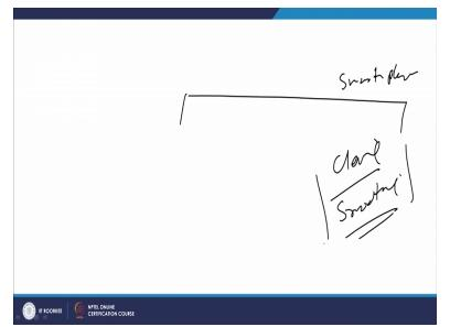
And there is one more like whatever the surface whose hardness to be checked that must be smooth, plain and free from impurities like oxides. Because if the oxides are present oxides may be harder for softer in so accordingly it will be decreasing or increasing the size of impression and that indirectly be giving the wrong value of the hardness. So, cleaning and smoothening of the surface whose hardness is to be checked is important (**Refer Slide Time: 28:20**)
