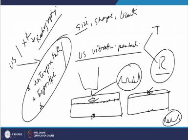
These are the ultrasonic testing and X-ray testing which is also called like radiography testing. So, the basic principle of the ultrasonic testing we have already talked that the ultrasonic vibrations can penetrate the metals and whenever they come across any medium or interface due to the change of the medium then these vibrations are reflected. So, basically there are two approaches one is the transmission approach and another is a reflection approach.
