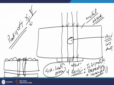
The radiography is the another method radiography is the another method which can use the Xrays or the gamma rays is mostly the X-ray method is very simple and very easy as compared to the gamma rays which is primarily used for thicker sections of a very heavy sections or assessing the soundness of the heavy sections. So, the property of these radiations is used in case of the soundness assessment is that these radiations actually can penetrate the metal.
