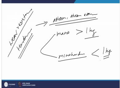
Apart from the bond strength another important property which is used for checking the wear resistance of the material is the hardness. This hardness indicates significant mechanical behaviour of the modified zones especially the resistance against the adhesion or abrasion, erosion. So, it is important to check the hardness of the modified zones. Basically there are two approaches one is called micro hardness and another is called micro hardness.
