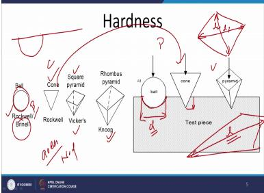
Considering this one if you see there are variety of the indenter which are used in different hardness tests like the ball, steel balls are used in case of the Rockwell hardness test for B scale and Brinell hardness test. Then cone is used in case of the Rockwell hardness test for C scale. Vickers hardness test uses the diamond in square shaped pyramid as indenter and Rhombus shaped pyramid is used for the Knoop hardness test.
