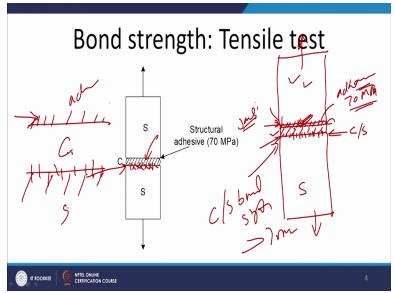
There is another indirect request method of the bond strength testing in this case like say this is the substrate and having the coating. So, we want to check the basically the coating substrate interface is strength, strength of this zone we want. But there is no direct measurement method so what we do will apply another structural material of the same as that of the substrate. And it will be joined with them coating itself using suitable adhesive.
