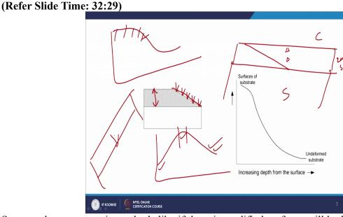
So, now there are certain methods like if there is modified surfaces will be like this is a substrate and this is coating. Since this coatings are very thin these coatings are very thin like maybe 200 to 500 micrometre. So, putting the intender in such a thin coatings will be difficult, so to measure the thickness variation from top to the interface what we do we make a slant surface like this. This may be 5 degree or 10 degree and then so we get the much wider length.
