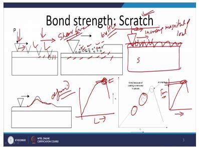
So, greater is the angle of the bend greater will be the bond strength that is how the indirect indication or the idea about the bond strength is obtained. Next is the scratch test method in case of the scratch test like say this is the substrate having coating like this. So, we apply one indenter, so, indenter is applied and it is moved indenter is applied with increasing magnitude of load so when it is moved the magnitude of the load is increased.
