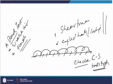
So, these are the two main factors one is application of the shear forces under the cyclic heating and cooling especially due to the differential thermal expansion coefficient can lead to the removal of the coating from the substrate. So, it is important to have that the coating is very formally bonded with the substrate. And that is why we need to check the coating substrate bond strength and therefore for checking the coating substrate bond strength.
