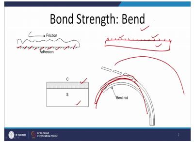
So, this is what has been explained in the like during the due to the shear forces if the forces are acting on to the shear force acting on to the coating then it can lead to the delimination from the surface of the substrate. In case of the bend test like this is a coating applied on to the surface of the substrate so the sample coated or the substrate coated, coated substrate will be subjected to the bending.
