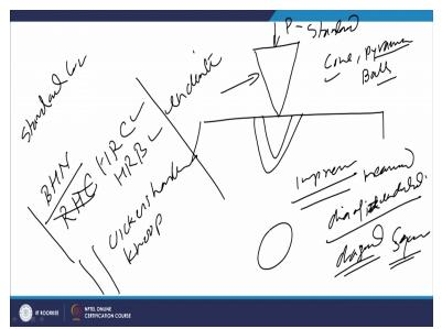
The basic principle of the hardness testing is simple where one had indenter of particular shape it may be in form of cone, pyramid it may in form of ball is used and one standard load is applied on to the modified surface and we will try to see how the surface of the modified surface is being affected because of this indenter. So, this is called indenter we apply one standard load and try to see how it is being affected.
