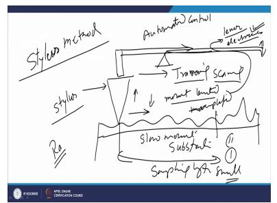
So, stylus based method in this case one pointed stylus small diameter is used and this is stylus is moved over the surface of the component whose roughness is to be measured. So, this is a stylus in very controlled way it is moved over the surface of the component. So, using automated control stylus is moved over the surface whose roughness is to be modified. So, this is the substrate and like say this is the modified zones.
