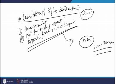
So, this we can considered as one limitation of the stylus based method because it takes time for quantifying surface roughness of the large surface area of the component which is to be characterized. So, I have said this is used for measuring the micro level surface roughness measurement. And if the nano level surface roughness is to be measured then there is another equipment which is atomic force microscopy.
