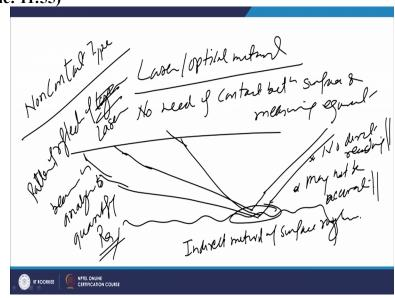
There is another category which is of the non contact type of the surface roughness measurement it uses the laser optical methods. In this case there is no need of contact between the surface and measuring equipment. So, this is one very good side and how does it work like the surface which is to be scanned or whose roughness is to be measured as directed with the beam of the laser. So, based on the kind of ups and downs present at the surface laser will be reflected in the different directions.
