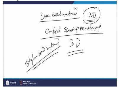
Then basically this laser based method gives us the 2D plot of the kind of the ups and downs which are present at the surface. There is there is one equipment which is called Confocal Scanning Microscope this also a laser based method but this is a confocal scanning microscope is also a instead of the two dimensional variation of the ups and downs present at the surface. This equipment gives a 3 dimensional variation or 3 dimensional patterns of the ups and downs present at the surface.
