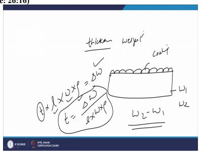
So, one is for thickness measurement we use the weight method. So, in this case the component which is to be whose surface is to be modified its initial weight is taken first and then after the modification again we take the weight of the component and difference of these two will be
