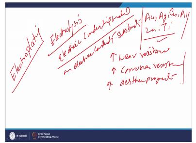
Now will take up the; another coating process which is basically electroplating process so, this is this process of coating is electroplating process it is based on the principle of the electrolysis. Primarily used for developing the coatings of the electric conducting materials on electric conducting substrate so means both coating material and substrate should be electrical conducting in nature.
