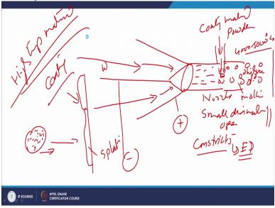
Which means there is one electrode and there is nozzle and this nozzle and arc is established between the electrode and the nozzle, so, electrode is primary tungsten which is connected to the negative terminal and the nozzle is connected to the positive terminal and then plasma forming gas is supplied so that the plasma is plasma forming gas passes through the arc and then this plasma is passed through the nozzle.
