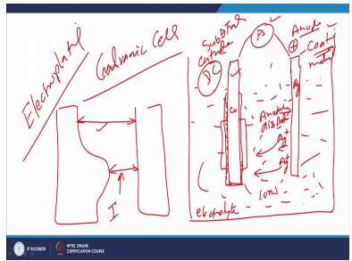
In this case basically the electroplating process uses the electroplating process is Galvanic cell for development of the coatings which is nothing a big tank full of the suitable electrolyte. So, here it is full of the electro light which is used as for completing the electric circuit between the substrate and the material to be coated. So, there are 2 members one is say good material to be coated coating material and this is substrate or the component on which coating is to be applied.
