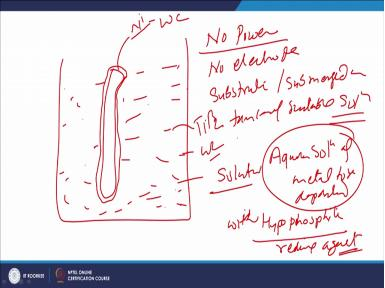
In this case there is no power requirement like in the electrolysis process where there was a; the flow of current and use of the DC supply and there is no electrode. Basically the substrate is submerged in the tank of suitable solutions where in the chemical reactions facilitate the development of the coating through autocatalytic chemical reaction process. So, in this case basically there is a tank having the solution like this.
