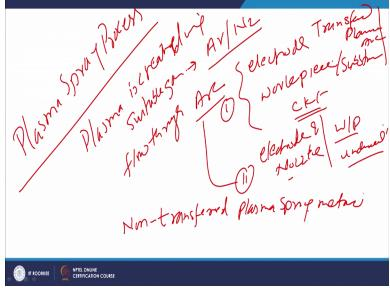
So, if you see the plasma spray process plasma spray process basically as we know that the plasma spray process basically the plasma is created using suitable gas like plasma forming gas which may be in form of Argon or the nitrogen. Now this plasma forming gas is allowed to flow through the arc. Now this arc established between the electrode and work piece or the substrate. This is case of the transferred plasma arc or the arc can also be established between the electrode and the nozzle.
