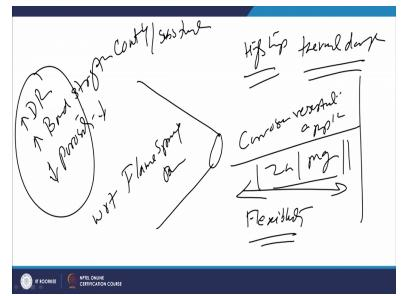
So, because of high temperature there is will be there will be the tendency for thermal damage to the material which is been deposited. But since in this case the work piece is the substrate is independent of the electric circuit and arching is taken place between the two wires only. So, there is a good flexibility as far as standoff distance between the arc spray nozzle and substrate is concerned.
