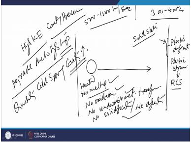
So, if you see this process is characterized as a very high kinetic energy coating process because the particles attain very high velocity of 500 to 1500 meter per second and the rise in temperature of the particle is also not the high as the gas temperature. The hot gas temperature is limited to 300 to 400 degree centigrade. So, if we see the particles which have not been heated too much higher temperature when they are accelerated to very high velocity after the impact they get flattened.
