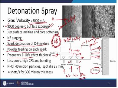
Now we will see the second process this is called detonation spray process in this; this another high velocity is spray process where in the velocity of the gas is too high like 3000 meter per second the temperature is 3000 degree centigrade. But since the velocity is very high and that is why we exposure of the material coated is for very less time and since the time is less at high temperature time of exposure at high temperature is less.
