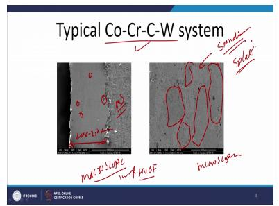
In the next slide always showing typical HVOF coatings of the Cobalt Chromium Carbon Tungsten system and if we see this is the macroscopic image of HVOF coatings of this material, this is the Cobalt based material which of these very good abrasion resistance as well as corrosion resistance. And we can see here this coating thickness is about the 200 to 250 micrometre. And this is a coating is developed on the surface of the mild steel to investigate what kind of the wear resistance.
