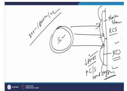
And then since the velocity of the powder particles which is a attended during the spray process is very high and that is why is this powder particles where just the surface has been brought to the molten state and the core has been soften and when the impingement of these particles happened at very high velocity then it will be leading to the flattening with the very of firmness and with very soundness and it will be leading to the reduced pores.
