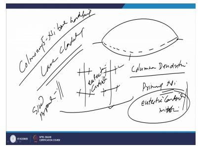
And typical materials like on columnoy there is one nickel base hard facing material are the cladding of this is deposited using the laser. Laser cladding of the columnoy and whenever it is it is just for an example whenever columnoy 5 coating cladding applied using the laser. It results in coating substrate interface results in columinor dendratic structure which is primarily made of the primarily it is nickel and between the dendratic forms we have the eutectic carbide mixture.
