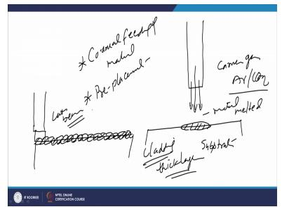
So there are there two variants associated with this process here the laser beam is directed on to the surface of the substrate. So, this will be facilitating diffusion of very thin layer of the substrate. Here the descent and to apply the material for surface modification there are two variants where in the coaxial feeding of material means material in powder form is fed along with the laser itself on to the surface of the substrate.
