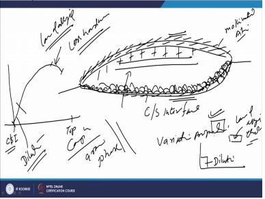
So, on approaching for from like say this is the cladding substrate interface. Initially normally we get the planar structure next to that it is very thin. This is a planar structure sometimes it is absent also. There after we get very fine cellular structure width very fine. There after we get another layer of the columner dendratic structure. These structures are very, very fine, columner dendratic structure.
