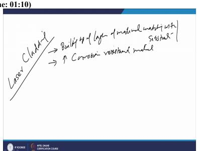
So the process is used so the process is laser cladding you know the cladding is used for depositing a thick layer of the material to be deposited on to the surface of the substrate for surface modification. And this can be used for building up of a layer building up of layer of the material matching with the substrate this one possibility. So, this can be machined out and we can regain the required size and shape.
