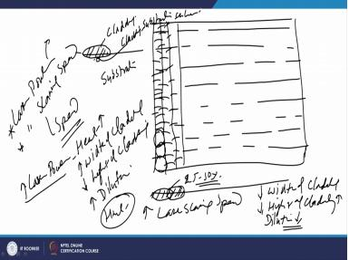
And whenever it is applied how it is applied because the laser beam diameter is very small and if the large areas to be scanned then say we are using the pre-placement technique than the material to be applied will be spread all over the surface area either in form of the paste or by the thermal spraying. And then after applying the material on the surface of the substrate the laser beam will be scanning the surface one by one like this.
