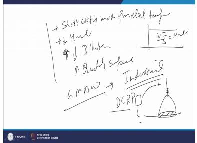
So, whenever short circuiting mode of metal transfer is used it helps since it is achieved using the minimum possible heat input and therefore it helps in reducing the dilution tendency. It decreases the dilution and the protective environments of the inert gases are inactive gases helps in developing quality weld surface. So, that is why GMAW variant is found extremely good for developing the weld surfacing at the industrial level for production of the many useful components.
