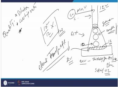
And we have seen that the performance of the quality of the surfacing is affected by the dilution and the cooling rate which is experienced by the weld metal during this solidification. And apart from this there can be other compositional degradation during the surfacing. So, what are those I will talk little bit about that. Let us say there is one material which is to be deposited on the surface of the substrate to achieve the required set of the properties.
