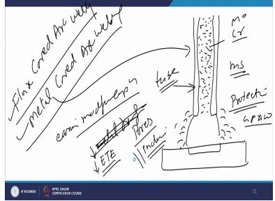
There is another variant of the gas metal arc welding process which is called flux cored arc welding or there is a one more variant which is called metal cored arc welding. So, idea behind this process is simple where we use one tubular electrode. So, there is a tube and inside that tube we feel in the flux. Flux may be with various types of the carbonate, Sodium, Potassium and line saw dust etcetera. These are basically this flux when the arc is established between the tube and the substrate.
