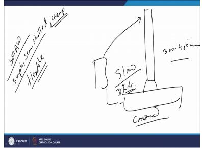
So, let us say when the SMAW process is used for Weld surfacing the process is very simple even semi skilled worker can apply this the process used is very simple equipments to the processes cost effective and cheap. It is very flexible it can be applied and you have not necessary to use and up use it in factory environment. But there are certain issues like a SMWA process uses one consumable electrode which is generally of likes in 300 to 400 mm length.
