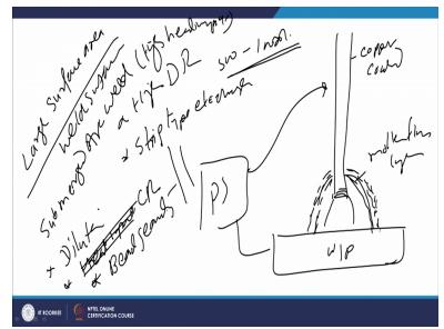
So, there are other alternatives as far as the under the conditions when large surface areas need to be modified by the weld surfacing. There are other options which are available like submerged arc welding. This is known as high heat input process and therefore allows us the very high deposition rate. All like current values maybe like 500, 1000 amperes so this is very good side and it permits the higher deposition rate.
