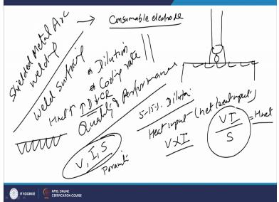
And now we have also talk little bit about the shielded metal arc welding processes. So, this group of the processes where the welding process are used to deposit the bead on plate these are called weld surfacing where bead on plate is deposited. In case of the shielded metal arc welding processes one consumable electrode is used and arc is strike between the electrode and work piece.
