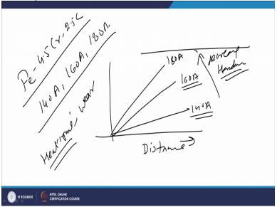
We will take up one example where in like iron 4.5% chromium and 2.5% carbon was used for this is a typical iron chromium and carbon hard facing systems. So, in this case if say the hard facing over deposited using the three level of current like 140 ampere, 160 ampere and 180 ampere and then try to see how does the behaviour of the hard facing change as a function of the current and what we see that that like if such kind of the hard facings are tested by the abrasive to wear test.
