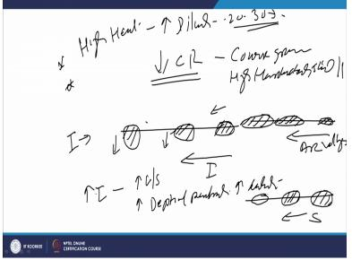
So, since the process high heat Input and their dilution levels are very high like 20, 30% so there will be lot of composition on modification of the world surfacing which will be developed by this process. But since high heat input allows the law coverage of the large surface areas and very fast pace because of the higher position rights which are possible. Further high heat input also reduces the cooling rate reduction in cooling rate will be leading to the course grain structure.
