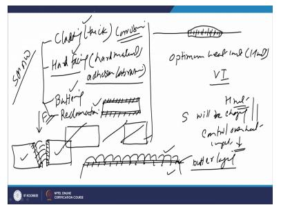
So that the good bond between the bead and the substrate can be created. Like if the heat input is very less than metal will simply be spreading over the subs over the surface of substrate and not very good metallurgical bond will be created. So, in this case poor bonding may lead to the denomination of removal of the bead. If the melting of the substrate is up to sufficient depth then it will be leading to the good metallurgical bonding.
