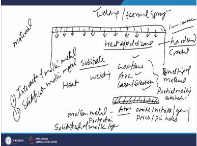
Where surface layer is developed or either using the welding or thermal spray based processes. So, using both this process completely thick layer ranging from 10 to 10's of 1000's of micrometer is developed. Like the welding is used for the claddings and the layers of the thickness greater than 1 mm or 1000 micrometre while recruiting is normally used for lower thickness is like a 10 to 1000 micrometre.
