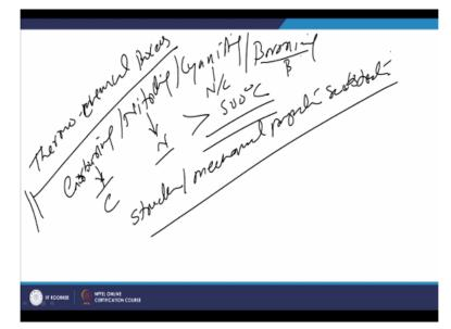
And there is no damage to the mechanical properties of the substrate as well as and because of the lower temperature will see then no distortion and the dimensional variation related issues. So this category of the processes are good in that way, then another category of the processes thermochemical processes. So in this category we have the carburizing, nitriding, cyaniding, boronizing.
