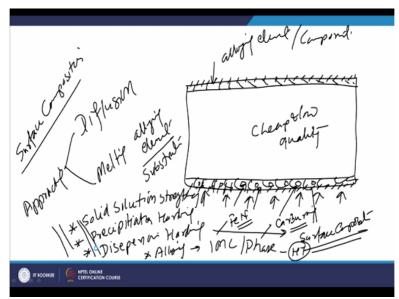
So in this broad category of the surface modification techniques where surface composition is modified to get the required set of the properties, you know in the surface engineering we normally use the main component of somewhat cheap and low quality material which is able to take the major load of the system. But the surfaces properties are not good enough to perform the expected functions for longer time.
