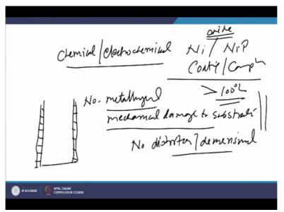
So 1 method is where the chemical or electrochemical reactions are used. So this kind of method is used for depositing the core in Nickel or nickel phosphate coating and modifying the composition of the surface layers. So in this case the temperature of the substrate is maintained well below the 100 degree centigrade. So in this category of the processes is the temperature is maintained within 100 degree centigrade.
