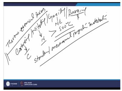
In this processes temperature used is greater than 500 degree centigrade and because of this there is every possibility are change in the structure and mechanical properties of the substrate. So the substrate characteristics and properties are expected to get modified when the components process through the thermochemical processes because they are performed at high temperature for modifying decomposition of the surface and near surface layers.
