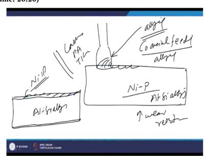
So this arc or laser will be melting the base metal at the same time through the external source the element to be introduced is fed in this zone. So melting of this one is also facilitated, there can be coaxial feeding of the alloying elements which are to be introduced at
