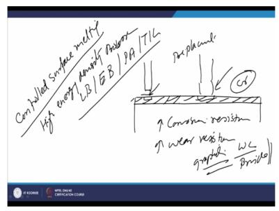
There is another approach where in the controlled surface melting is used using the high energy density processes like we can use the laser beam, we can use the electron beam or we can use plasma or even the GTA or TIL R is also used. All these are non consumable and processes where the consumable is fed in the heating zone if we want to apply or we want to deposit anything on to the surface.
