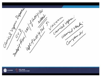
In this presentation we will be talking about the 2 surface modification processes, 1 is the chemical vapour deposition and another is boronizing. So initially we will be starting with the chemical vapour deposition process, in short it is known as CVD and this is one of the most commonly used process for developing films or for surface modification of cutting tool inserts.
