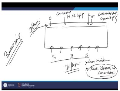
Now will take up the another process which is the boronizing, like we have seen earlier for modifying the chemical composition of the surface is we have seen so many processes like carbon is introduced in the processes like carburizing, nitrogen is introduced in case of the nitriding and mixture of both carbon and nitrogen is introduced in case of the carbonitriding and cyaniding.
