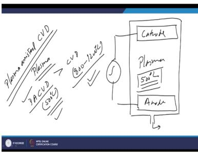
And advantage of this process is that it uses the plasma for absorption as well as a realising the required chemical reactions to form the compounds required. So in order to have for the plasma formation in this kind of system again will be using the vacuum system and apart from the things which are needed for the conventional chemical vapour deposition process it uses 1 anode and 1 cathode .
