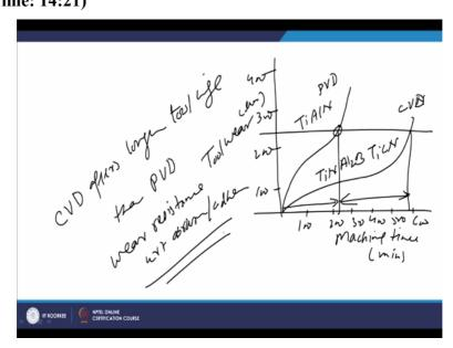
Especially the life of the component which is being modify say the cutting tool if in the x axis we have the machining time indicating the tool life in minutes and in the y-axis we have tool wear, so tool wear like say 100, 200, 300, 400 in micrometers and this is in cutting time. So her like say 100, 200, 300, 400, 500, 600 in minutes. So when we develop the coatings of the
