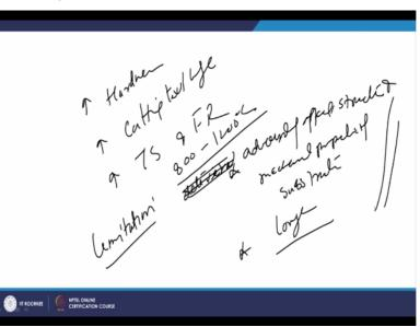
So in light of this if we see there are there are certain advantages related with this process that it is able to increase the surface hardness significantly which helps in increasing the cutting tool life especially with regard to the tool as well as it also helps in increasing the tensile strength and fatigue resistance of the component and the but apart from the positives associated with this chemical vapour deposition process there are few limitations.
