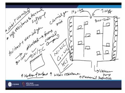
So what we use in this process basically 1 chamber which is made of the stainless steel is used is connected with the suitable vacuum pump for creating vacuum and then inside we have the suitable compartments for putting in the components to be modified for surface property enhancement. So here like since it is most commonly used for improving the properties of the cutting tool inserts will be placing the cutting tool inserts at the different compartments.
