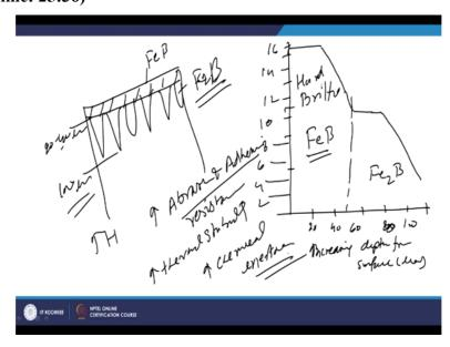
So increasing depth from surface in micrometre and in the y-axis we have the concentration of the boron. So obviously at the surface the concentration is very high. So like say the 16, 14, 12, 10, 8, 6, 4, 2, like this. So just at the surface this concentration is very high and then it will be somewhat lower then what will see or it will be reducing further.
