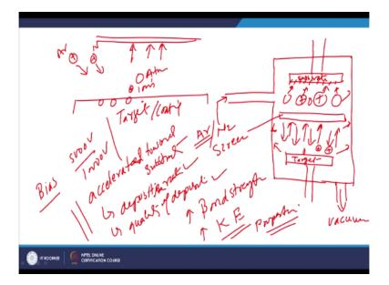
So that the high energy ions and the atoms can be for the accelerated towards the surface of the substrate. So these are the important features related with this process. So now will see like this the ions of the argon or the nitrogen are directed at high with high energy on the substrate or on to the target which is basically coating material which is to be applied. So with these impact and will be producing some of the ions of this target material and the atoms are also removes.
