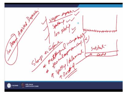
Bias is used of the sufficient distance so that these can be accelerated towards substrate anal to have with bond strength as well as sufficient deposition rate. Now will be what is the another very useful surface modification technique by changing the chemical composition, that is the iron beam assisted deposition. So as we have seen in case of the vapour deposition and sputtering in both these cases are iron plating.
