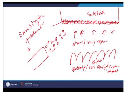
The cracking tendency and brittleness tenancy is reduced when iron beam assisted deposition is used. So the general principle of this process is what substrate and the suitable source of the target material which is to be deposited and maybe in case of the sputtering, in case of the ion plating or in case of the vapour deposition. These target material will be providing the either atoms, ions, vapours which will get deposited, which will move towards the substrate.
